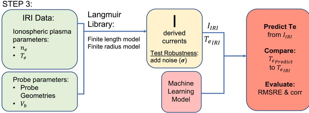
**Figure 4.** Vizualisation of Step 3: Use another data source (here from IRI) (green box) to derive measured currents (yellow box) to test the machine learning model on (pink box). Evaluate again the inferred temperatures compared to the ground truth (here IRI) temperatures (red box). To test the robustness, add different noise levels to the derived current (yellow box), according to equation 9.
