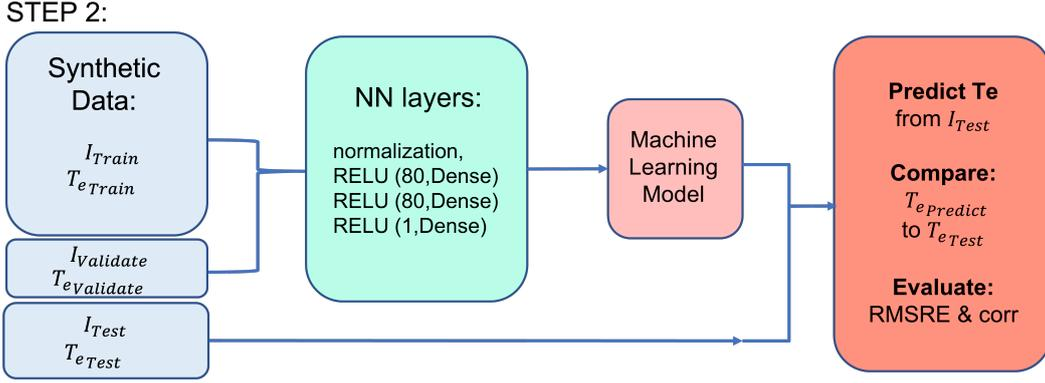
**Figure 3.** Visualization of Step 2: Use the training and validation data (blue) from Step 1 to train a NN (turquoise box) and save a machine learning model (pink box). Use then the test data current (blue box) from Step 1 and apply the machine learning model (pink) to it. Finally, evaluate the performance of the inferred temperatures compared to the ground truth temperature (red box).
