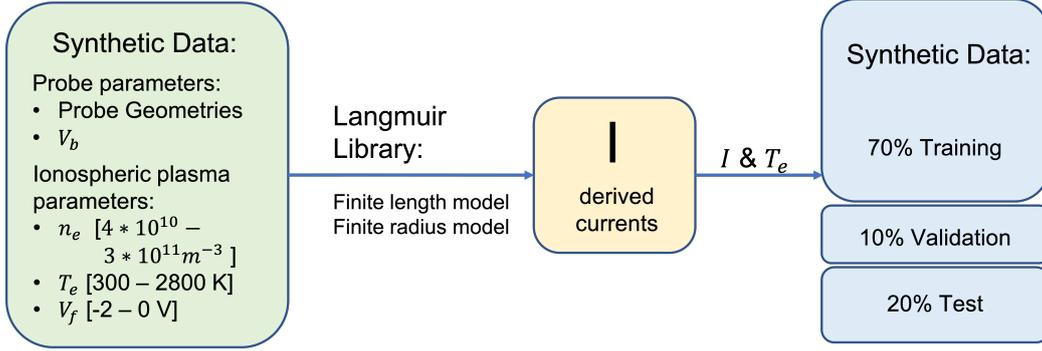
**Figure 2.** Visualization of Step 1: Construct the synthetic data set (green box), to then derive currents (yellow box) using the Langmuir library finite length and finite radius model and creating the combined synthetic data set of ionospheric plasma parameters and collected currents (blue box).
