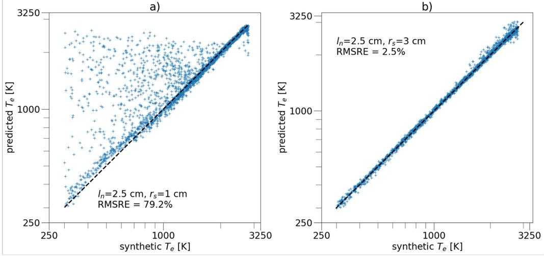
**Figure 7.** Setup 3), four cylindrical Probes and a spherical probe: Predicted temperatures versus synthetic temperatures of the test set are shown in form of scatter plots in panel a,b. Probe geometry and RMSRE are reported in the plot texts.
