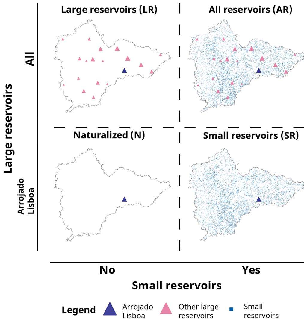
**Figure 2.** Visualization of the modeled scenarios design: Large Reservoirs (LR), centralized reservoirs only; All Reservoirs (AR), centralized reservoirs and DRN; Naturalized (N), Arrojado Lisboa only; and Small Reservoirs (SR), DRN and Arrojado Lisboa only.
