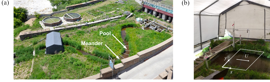
Figure 1. (a) The OSL facility, with the locations of the two ROIs (meander and pool) indicated by arrows. The tent, shown here at a downstream location, is deployed over the ROIs in the present experiments. (b) The traversing system holding the camera used for free surface imaging, indicating the approximate location of the FOV in the meander and the 2D coordinate system.
