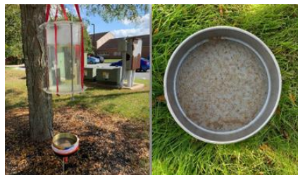
Figure 2. Aggregates stability analysis. Displayed is the rain stimulator whose mechanism actions is equivalent to a thunderstorm ((Moebius-Clune, 2017).
