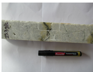
Figure 26. a: Smoky quartz vein ( V2a) in tonalite with 26.82 g/t in core drilling hole FNDC012 (PDY005); b: Sulphide hosted in the Smokey Quartz Vein (V2a), metallographic microscope; c: quartz veinlet stockwork (V2b) in tonalite with 65 g/t in core drilling hole FNDC012@40.80m
