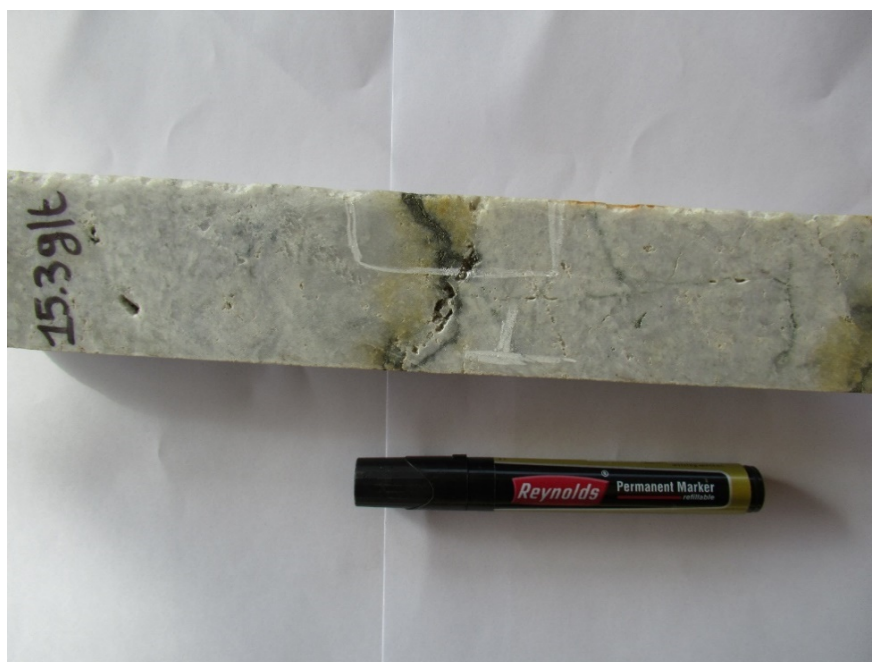
Figure 26. a: Smoky quartz vein ( V2a) in tonalite with 26.82 g/t in core drilling hole FNDC012 (PDY005); b: Sulphide hosted in the Smokey Quartz Vein (V2a), metallographic microscope; c: quartz veinlet stockwork (V2b) in tonalite with 65 g/t in core drilling hole FNDC012@40.80m
