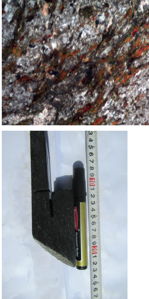
Figure 20: a: Photograph of diorite (TDY013) in drill hole FNDC008@103.3m, showing Shearing foliation S3, Contact Diorite / Sandstone b: Shearing filiation S3 in (TDY013) in drill hole FNDC008@103.3m, metallograhic microscope
