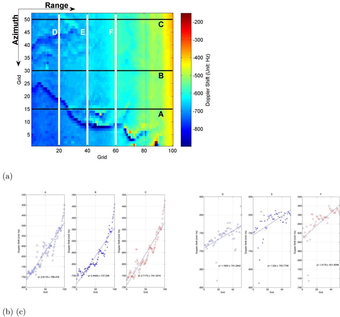
**Figure 1.** The linear trend of the Doppler centroid frequency  $f_{DC}$ . (a) The  $f_{DC}$  image derived from the Environmental Satellite (ENVISAT) advance synthetic aperture radar (ASAR) mapping on 07/14/2007 at Hangzhou Bay, with three profiles A, B and C along the range direction and three profiles D, E and F along the azimuth direction.. The linear trends of the profiles along the (b) range and (c) azimuth directions.
