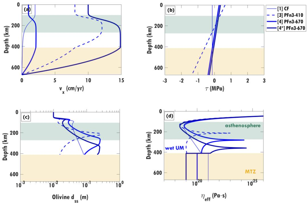
**Figure S8.** The (a) four flow configurations plausible for wet (1000 ppm H/Si) upper mantle and their associated (b) stresses, (c) grain-sizes, and (d) viscosity structures. The corresponding plate speed and pressure gradient combinations used to produce such flows are shown in Figure 7b.2 (in blue rectangles).
