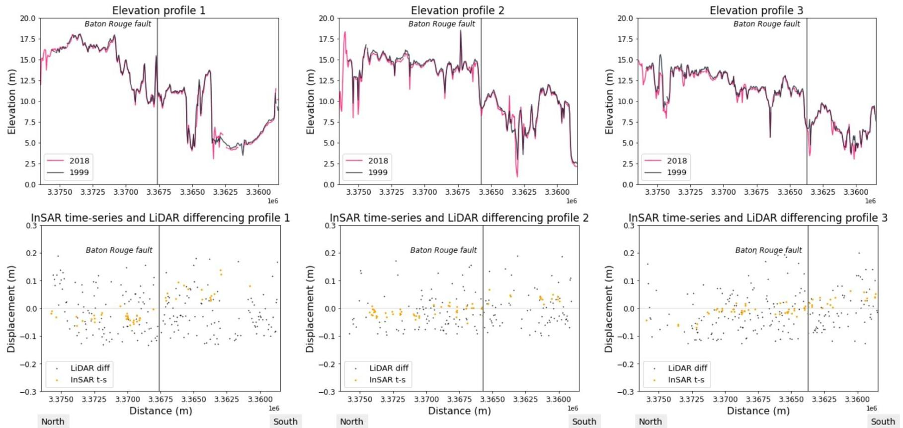
**Figure S1.** Comparison of elevations using the DEM from 1999 and 2018 in the upper panel and results from our methods along those profiles. For location of the profiles see Figure 1. For the upper profiles, data is averaged every 10 meters from the DEMs, and lower panel is averaged every 20 meters from the GCD results (Fig. 9) and the InSAR time-series for Sentinel-1 results (Fig. 5)
