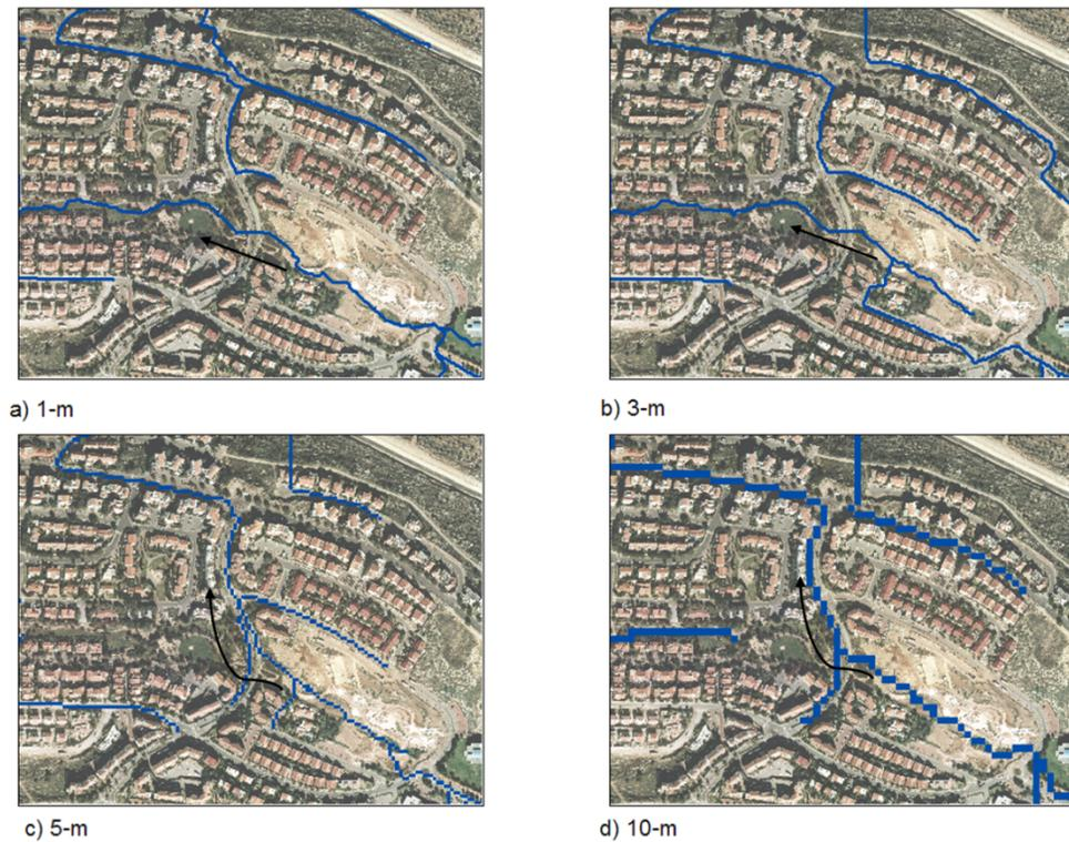
**Figure 3. Comparison of flow path delineation from DEMs that were derived directly from elevation data (contours, height points, etc.) using various cell sizes: a) and b) reproduce the actual flow path which is from east to west along the park, while c) and d) delineate a wrong north-flowing path**
