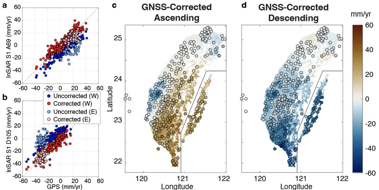
**Figure 2. Comparison of InSAR and GNSS velocities.** Comparison of velocities before and after correction for ascending (a) and descending (b) tracks. The red dash line in (a) and (b) represents a 1:1 ratio between GNSS and InSAR. W and E in (a) and (b) represent west and east Taiwan, respectively. Positive and negative values in (c) and (d) represent movement towards and away from the satellite LOS, respectively.
