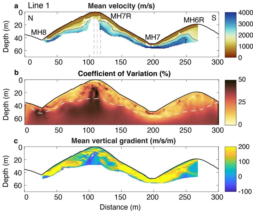
309 **Figure 4.** Results of Line 1 inversion using THB rj-MCMC (Huang et al., 2021). (a) Mean velocity model
