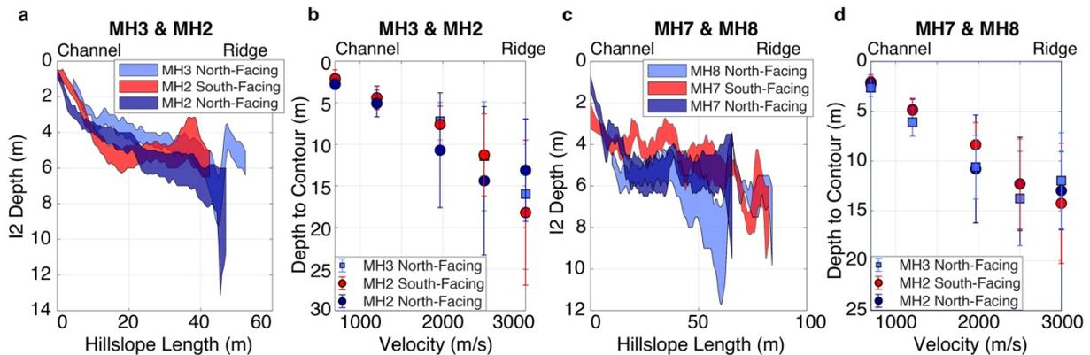
442 **Figure 10. Comparison of weathering thickness on north- versus south-facing hillslopes for Line 6**
