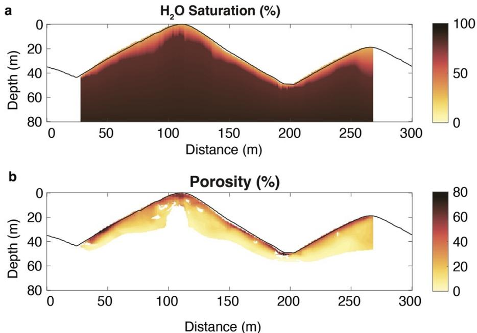
496 **Figure 12.** (a) A gradually increasing saturation model from 50-100% predicts (b) modeled bulk porosity
