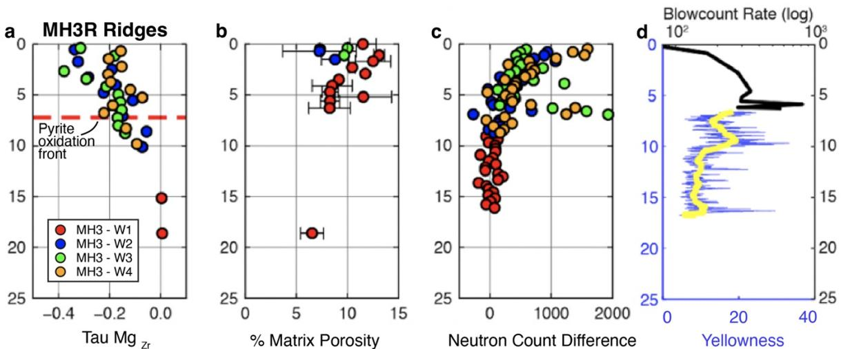
168 **Figure 2. Borehole data for the MH3R ridgetop in Line 6** (see Figure 1 for location). Data is from
