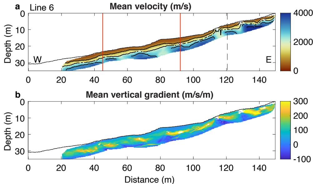
328 **Figure 5.** Results of Line 6 inversion. (a) Interpolated mean velocity model with contour lines at 1000, 2000,
