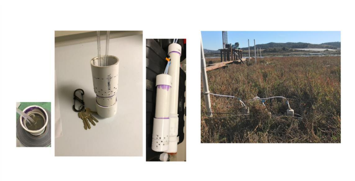
**Figure S3.** Photographs of sampling cups used in combination with a manifold pump and a field-base spectrophotometer to continuously measure  $NO_3^-$  concentrations in salt marsh porewater.
