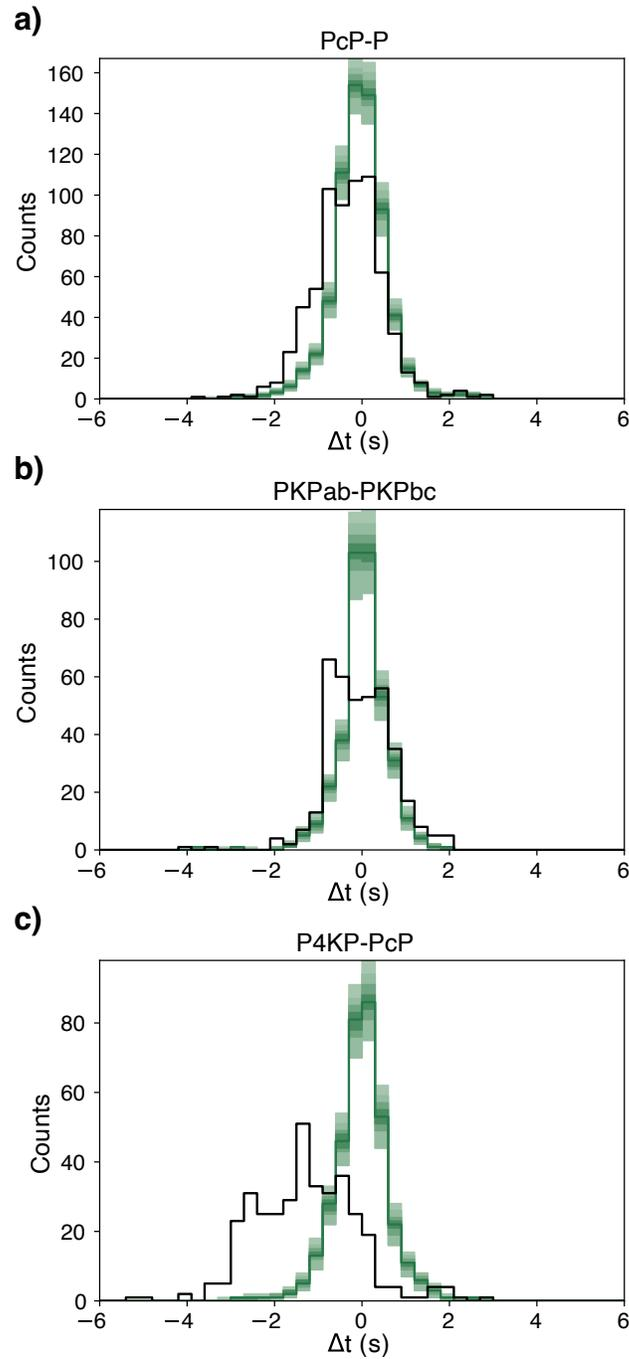
**Figure S2.** Travel time residuals for the 3 datasets used in this study. a) PcP-P, b) PKPab-PKPbc, c) P4KP-PcP Black histograms show the initial distribution of residuals, and green histograms show the deciles of remaining residual distributions after inversion.
