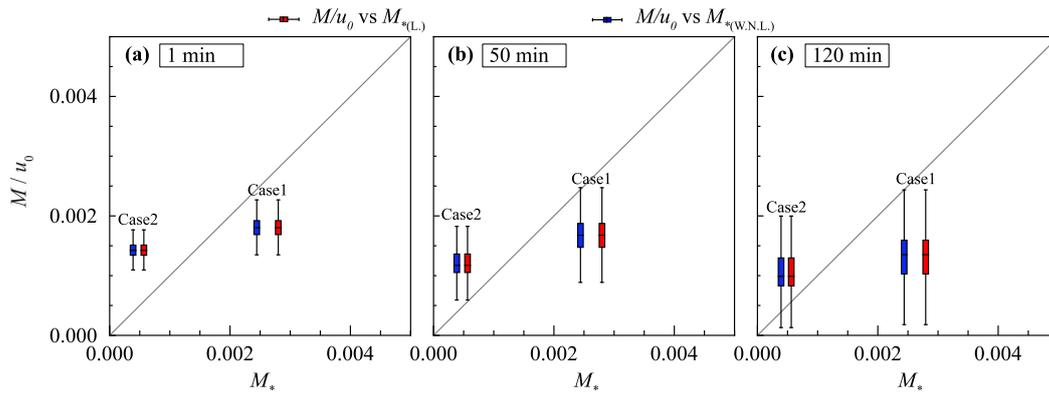
**Figure 13.** Relationship between migrating speed obtained by our method and migrating speed obtained by instability analysis.
