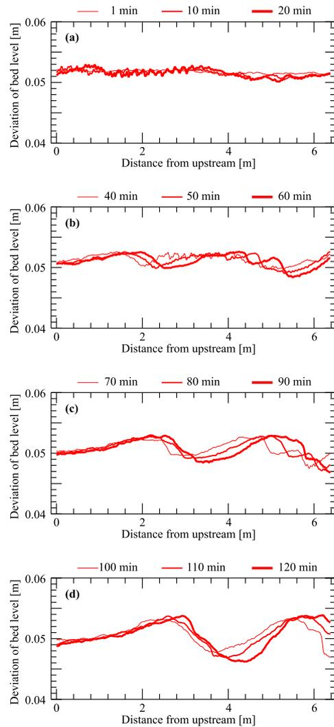
**Figure 4.** Longitudinal view of the measured bed shape: (a) Initial stage of the experiment, (b) occurrence of alternate bars, (c) intermediate stage of the experiment, and (d) final stage of the experiment.
