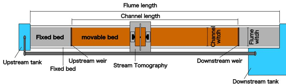
**Figure 2.** Plane view of the experimental flume.
