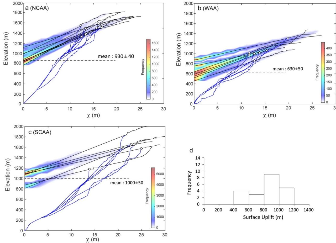
**Figure 7.** Modern longitudinal profiles and projections of the relict landscape (red segments) upstream of the highest knickpoints using  $k_{ref} = 0.45$  and the  $k_{sn}$  of the relict portion for the (a) NCAA, (b) WAA, and (c) SCAA sectors. Major knickpoints are marked with white circles. (d) Frequency diagrams of the magnitude of surface uplift for the different sectors.
