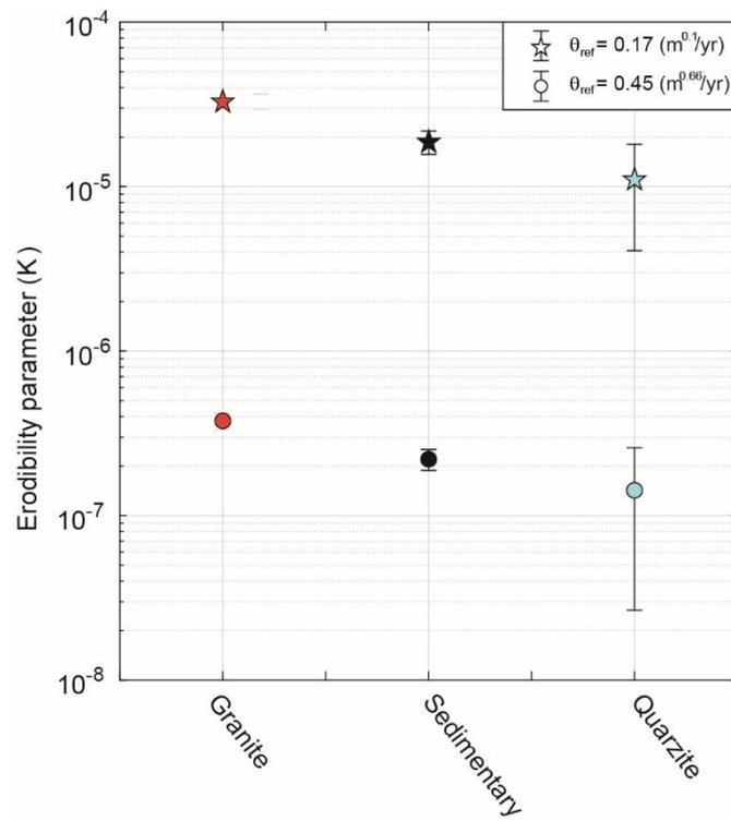
**Figure S5.** Rock-type versus erodibility parameter. Erodibility values were estimate from the forced linear regression between basin-wide denudation rates and basin-averaged  $k_{sn}$  using  $\theta_{ref}$  of 0.45 and 0.17 (mean value of concavity relative to uplifted relict landscape, Table S1), assuming  $n = 1$ .
