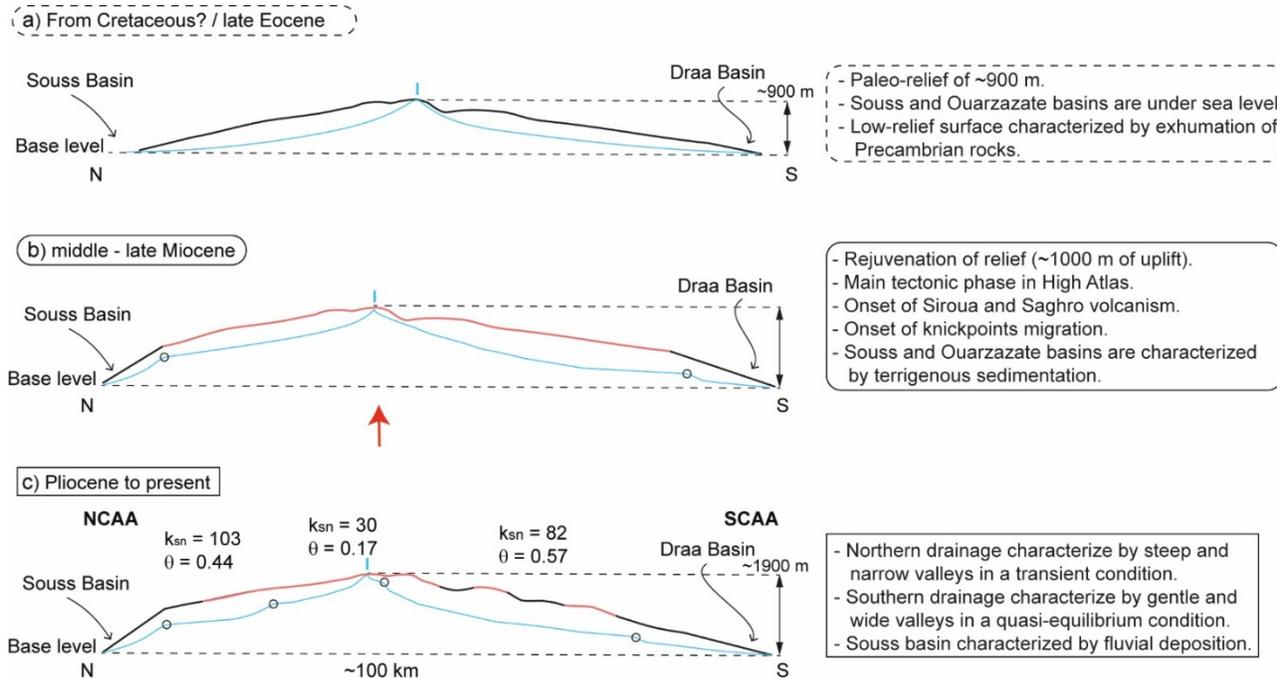
**Figure 13.** Conceptual model depicting the Anti-Atlas topographic evolution across the central Anti-Atlas. (a) Paleo-topography inferred until the late Eocene. (b) Topographic rejuvenation during the middle-late Miocene associated with the initiation of river incision and knickpoints upstream propagation. (c) Present-day configuration. Pink area describes the preserved relict landscape not yet rejuvenated.
