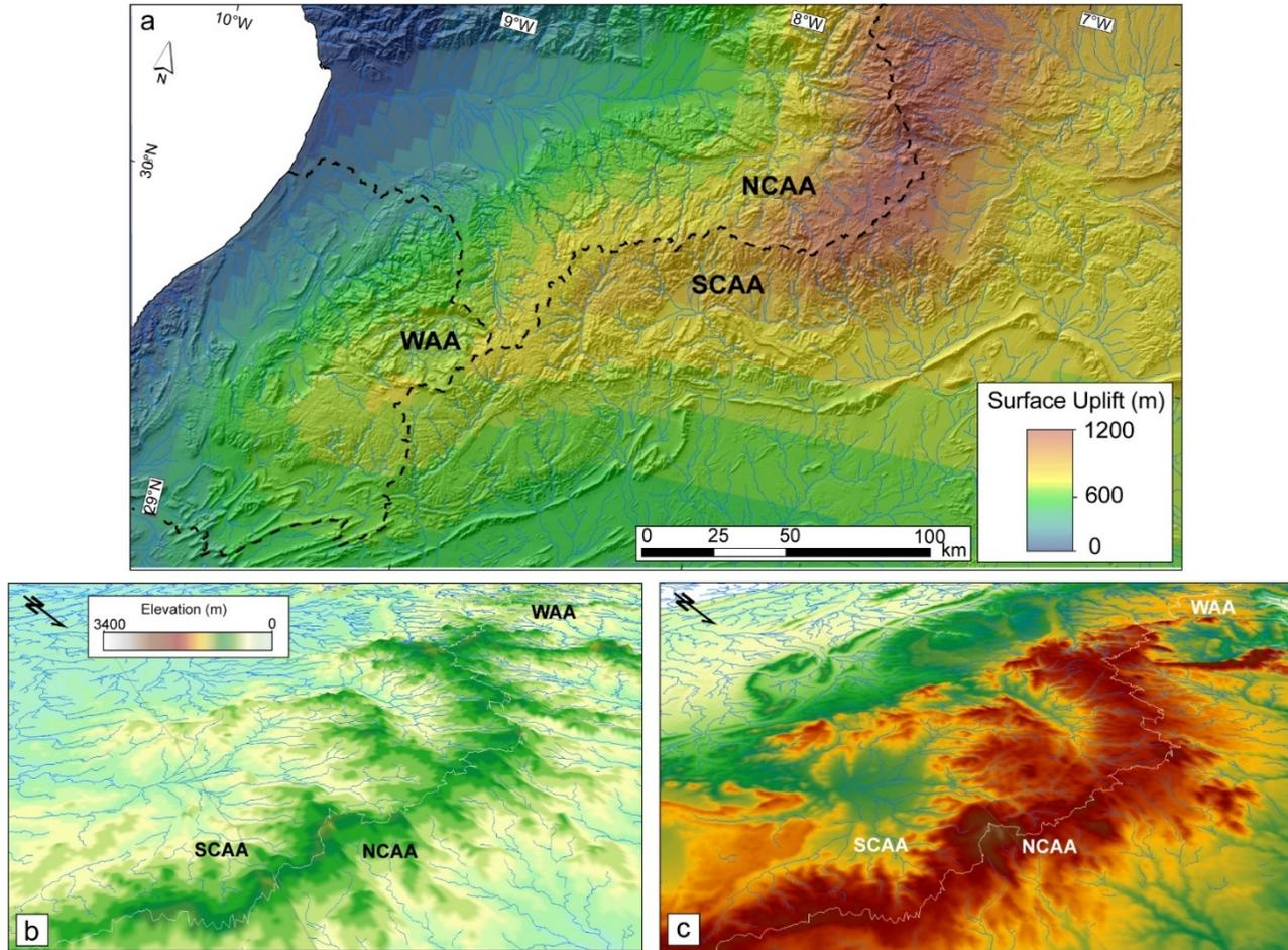
**Figure 10.** (a) Surface uplift ( $S.U.$ ) map. The base level is defined at the relict landscape boundary; values of  $m = 0.45$  and  $A_0 = 1 \text{ m}^2$  were used to calculate  $u^*$  (Equation 7). (b) Paleo-topographic reconstruction of the central and western Anti-Atlas. (c) Present-day topography of central and western Anti-Atlas.
