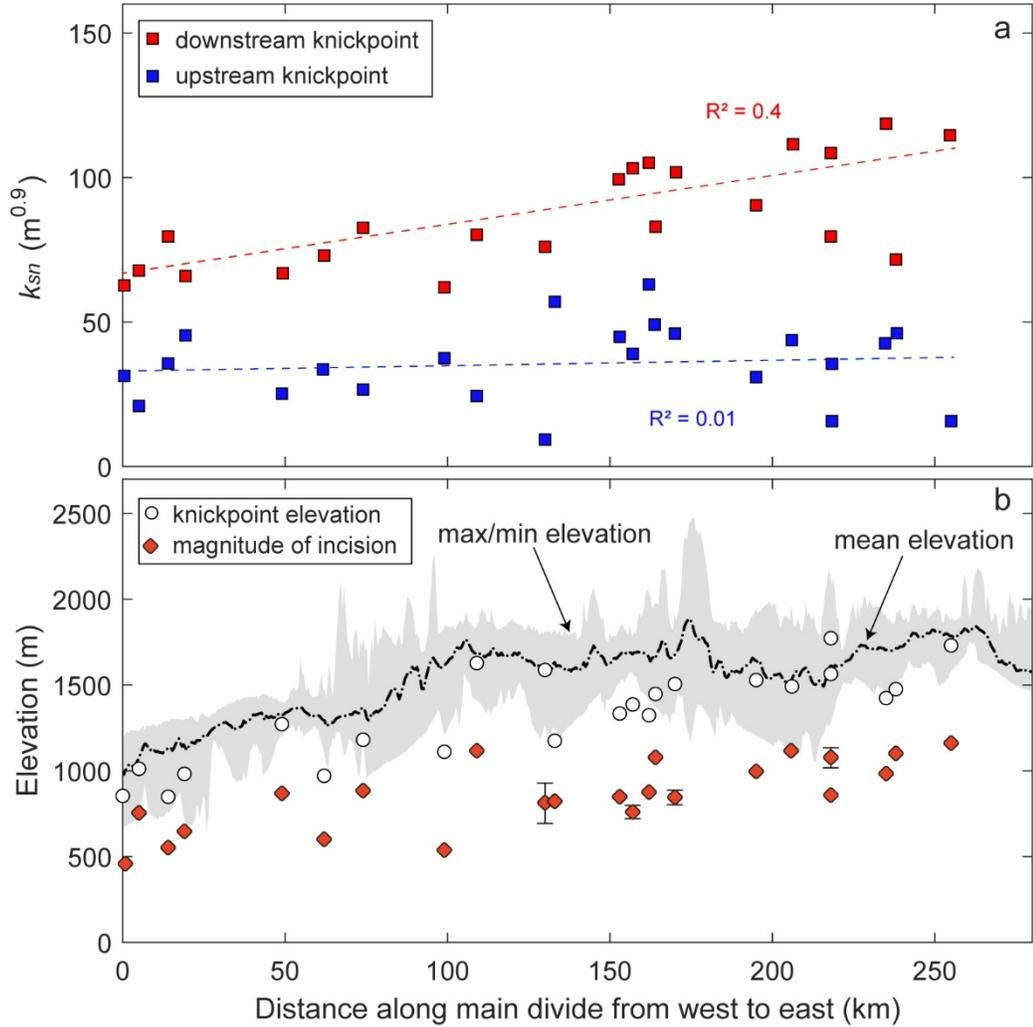
**Figure 9.** (a) Distance along the main drainage divide versus  $k_{sn}$  down and upstream of the non-lithological knickpoints. (b) Distance along the main drainage divide versus knickpoint elevation and estimated surface uplift values. The location of the swath profile is indicated in figure 2d.
