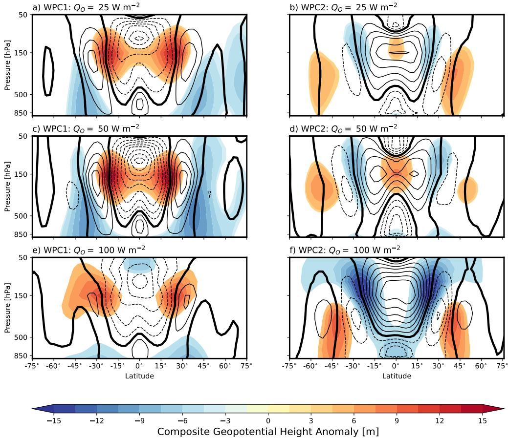
514 FIG. 8. Warm pool composites of geopotential height (shading) and zonal wind anomalies (black contours)
