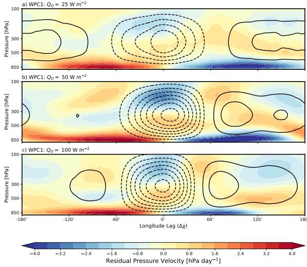
569 FIG. 10. Equatorial plane of WPC1 for the first baroclinic mode of the intraseasonally-filtered vertical velocity
