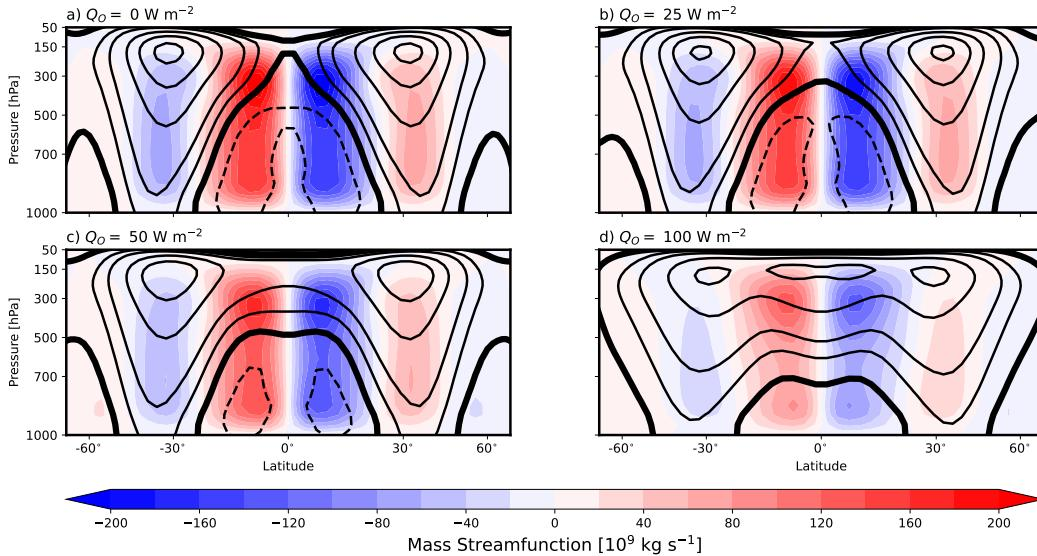
336 FIG. 2. Eulerian mass streamfunction (shading) and zonal mean zonal wind (black contours) for (a) the control
