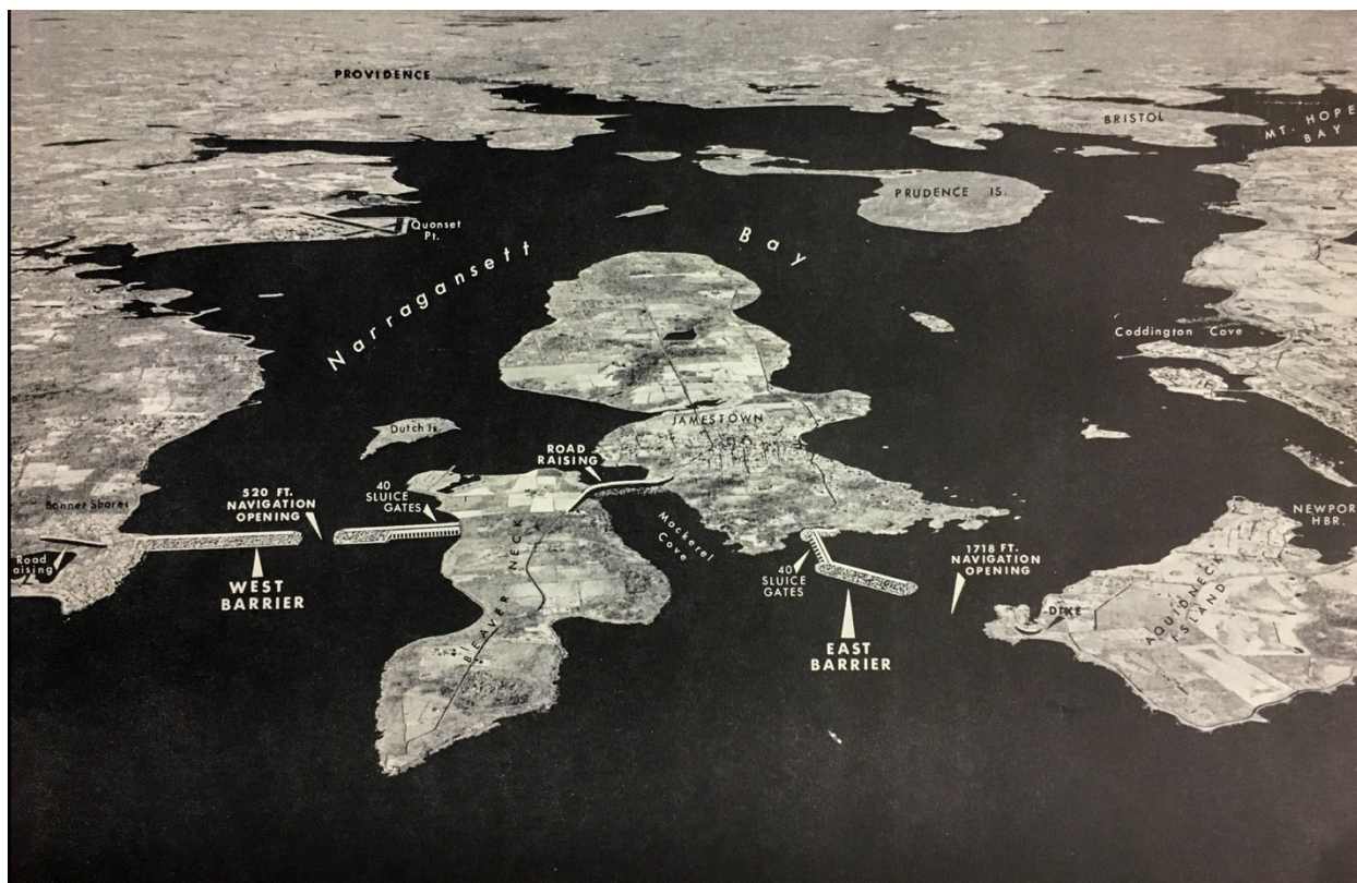
1187 Figure 2. Revised plans for the Narragansett Bay barriers, April 1964. Source: New England 1188 Division of the U.S. Army Corps of Engineers (Waltham, Massachusetts).
