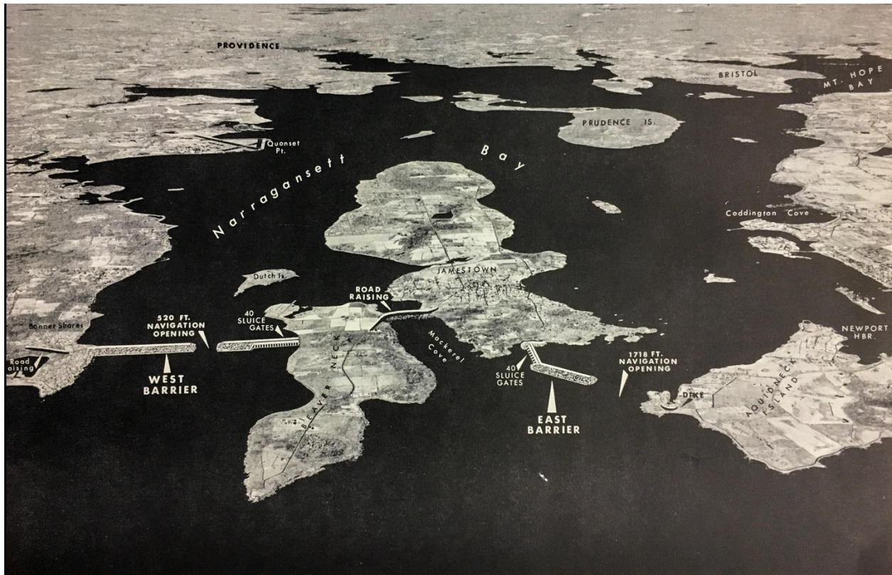
Figure 3. Revised plans for the Narragansett Bay barriers, April 1964. Source: the U.S. Army Corps of Engineers, New England Division. Waltham, Mass.
