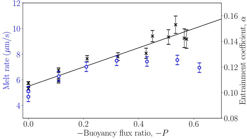
**Figure 3.** Measured melt rate (blue circles, left axis) and the entrainment coefficient estimated by McConnochie et al. (2021) (black crosses, right axis) plotted against the buoyancy flux ratio. Also shown is an empirical fit to the entrainment coefficient (black line, right axis) from McConnochie et al. (2021) given by  $\alpha = 0.105 - 0.75P$ .
