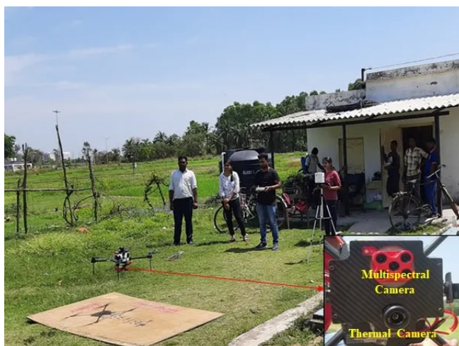
Figure 3. Aerial data collection using UAV equipped with multispectral (Micasense) and thermal camera (FLIR)
