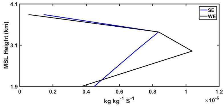
Figure 5: Rain evaporation rate ( $\text{kg kg}^{-1} \text{s}^{-1}$ ) for the events shown in Figure 2(a-b). The evaporation rate is calculated by using equation (1) from the microrain radar (MRR) measured values of raindrop size distribution parameters. SE and WE indicate strongly and weakly electrified.
