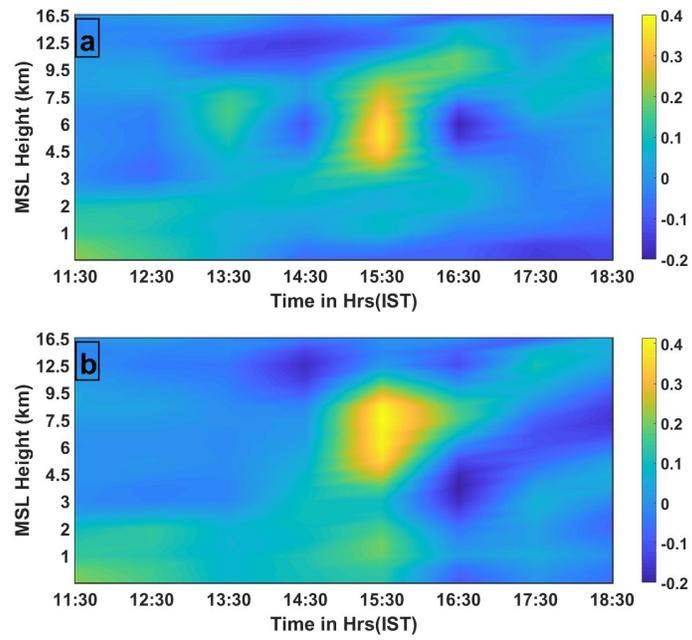
Figure 9: Results from real case simulation (13 May 2015)(a) Height Time Index of area averaged vertical velocity ( $\text{m s}^{-1}$ ) for wsm6 (b) same as (a) but for wsm6(M)
