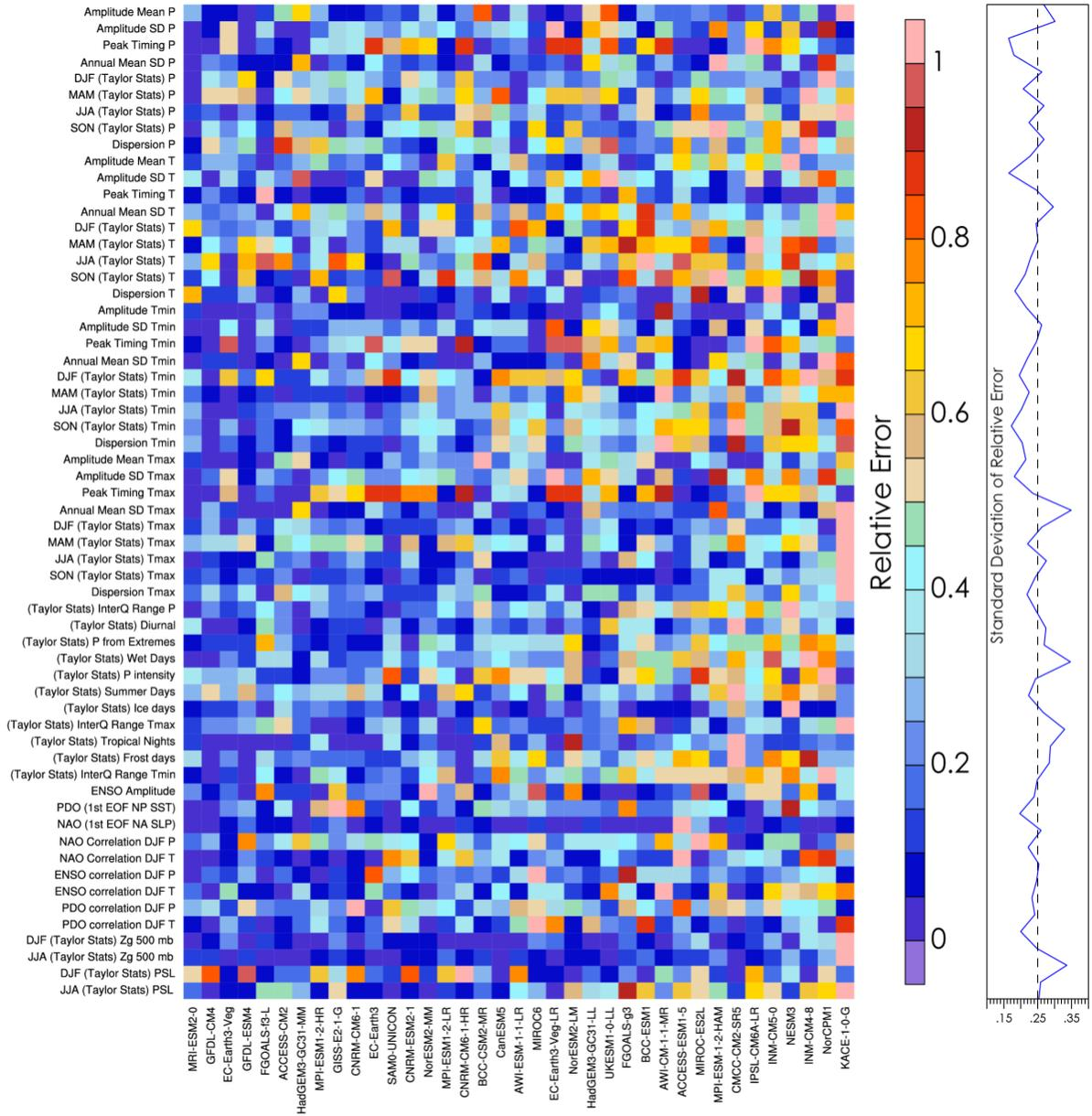
**Figure S1.** The unweighted relative errors of GCMs over the East. The left panel shows relative errors corresponding to each metric across all GCMs, and the line plot on the right shows the standard deviation of the relative error for each metric across all GCMs.
