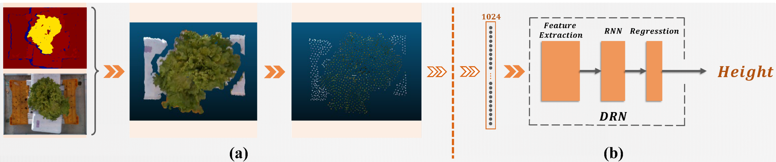
Figure 5. Overview. (a) Data and Data preprocessing, transform the give images into cloud point and downsampling. (b) Regressing lettuce plant height from single perspective sparse cloud point by our proposed DRN structure model
