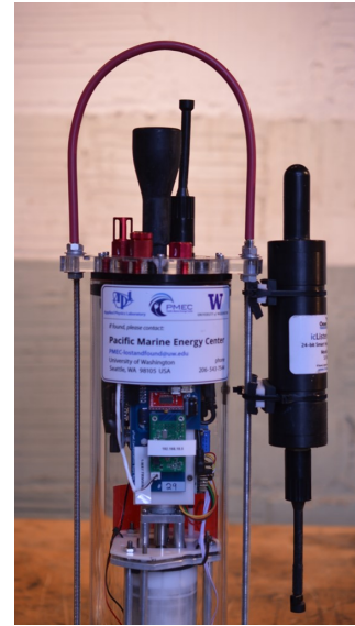
Figure 1: Hydrophone mounted to the side of the \mu Float.
