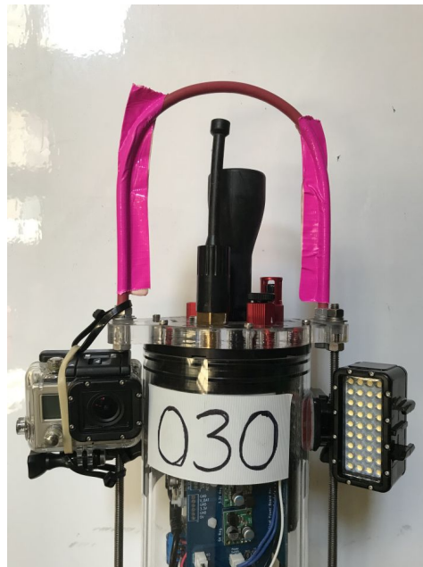
Figure 3: GoPro and supplementary light mounted to the side of the \mu Float.
