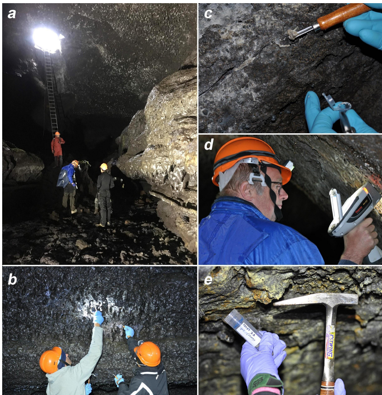
Figure 3. Sampling strategy. (a) Cave entrance to cave H, 12 m below ground. (b) Sampling in pairs: one sampler and one assistant handling cleaning and handing over of tools. (c) Biological sampling (step 2): scraping mats from the cave wall. (d) Handheld XRF measurements of cave wall (step 4). (e) Substrate sampling with a geological hammer and Falcon tube (steps 3 and 5).
