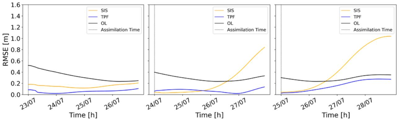
**Figure 10.** Hourly Root Mean Square Error (RMSE) time series. The black line represents the RMSE of the OL, the blue line the TPF-based RMSE and the orange line the SIS-based RMSE. 3 different assimilation cases are plotted: 07/23 00:00, 07/24 00:00, and 07/25 00:00.
