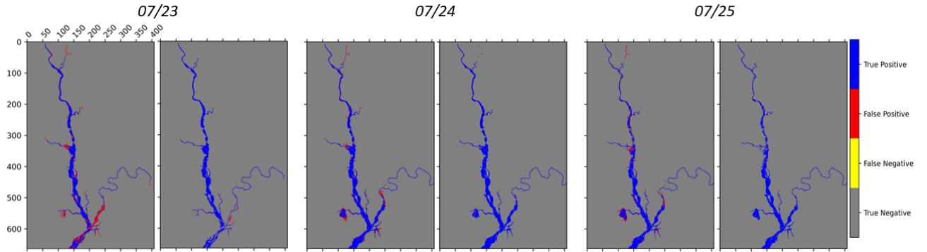
**Figure 4.** Contingency maps of the Open Loop (left) and after the assimilation (right) for three different assimilations at time 07/23 00:00, 07/24 00:00, 07/25 00:00. Red pixels correspond to over-prediction (false positives) errors, yellow pixels to under-prediction (false negatives) errors, pixels correctly classified as not-flooded are in grey and when the contrary occurs pixels are in blue.
