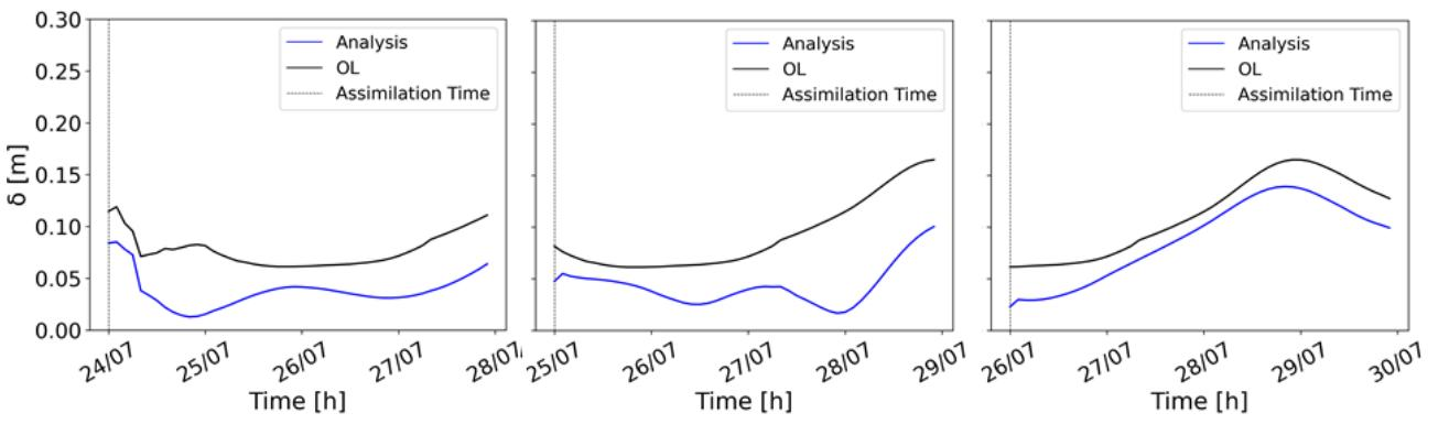
**Figure 8.** Hourly time series of the RMSE. Black line refers to the OL and blue line to the analysis results after the assimilations of 3 different images (07/23 00:00, 07/24 00:00, and 07/25 00:00).
