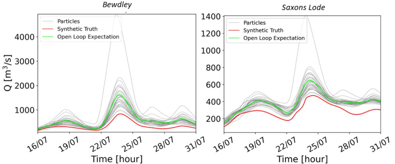
**Figure 11.** Discharge time series ensemble at Bewdley (on the left) and at Saxons Lode (on the right). The OL particles are represented with gray lines, the synthetic truth is represented by the red line. The OL expectation is in green. In this case, the ensemble is markedly biased; the synthetic truth falls outside the ensemble range most of the time.
