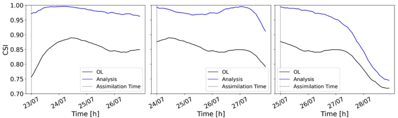
**Figure 5.** Hourly time series of the Critical Success Index of the Open Loop (black line) and Tempered Particle Filter analysis (blue line) due to the assimilation of 3 different images: during the rising limb (07/23 00:00), at the peak (07/24 00:00) and during the falling limb (07/25 00:00).
