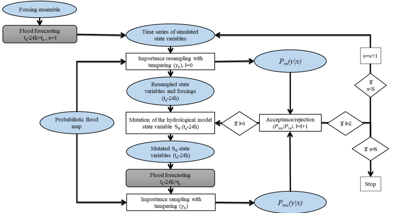
**Figure 2.** Flow chart of the DA framework where synthetic probabilistic flood maps are generated from flood extents, derived from a truth run, and assimilated within the same flood forecasting model. The flood forecasting model is represented with a grey rectangle, mathematical operations with a white rectangle, state variables, input and observations with a blue ellipse.
