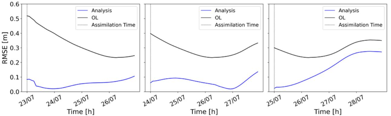
**Figure 7.** Hourly time series of the standard deviation of the errors due to the assimilation of 3 different images: 07/23 00:00, 07/24 00:00, and 07/25 00:00. The standard deviation of the errors as difference between the OL and the true water levels (black line) and as difference between the analysis expectation and the true water levels (blue line).
