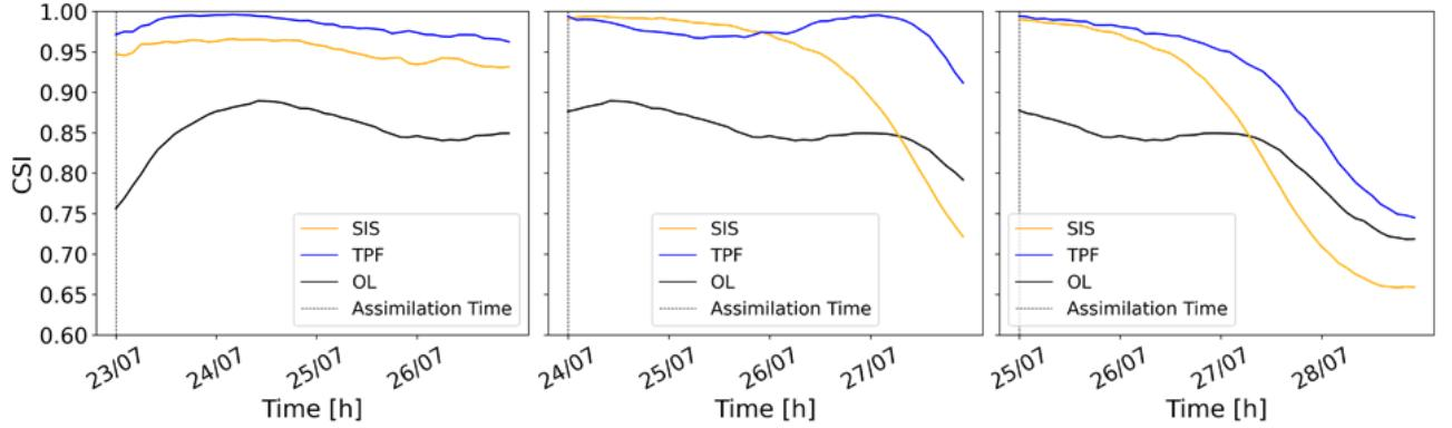
**Figure 9.** Comparison of the hourly time series of the Critical Success Index of the OL (black line), TPF analysis (blue line) and SIS analysis (orange line) due to the assimilation of 3 different images: 07/23 00:00, 07/24 00:00, and 07/25 00:00.
