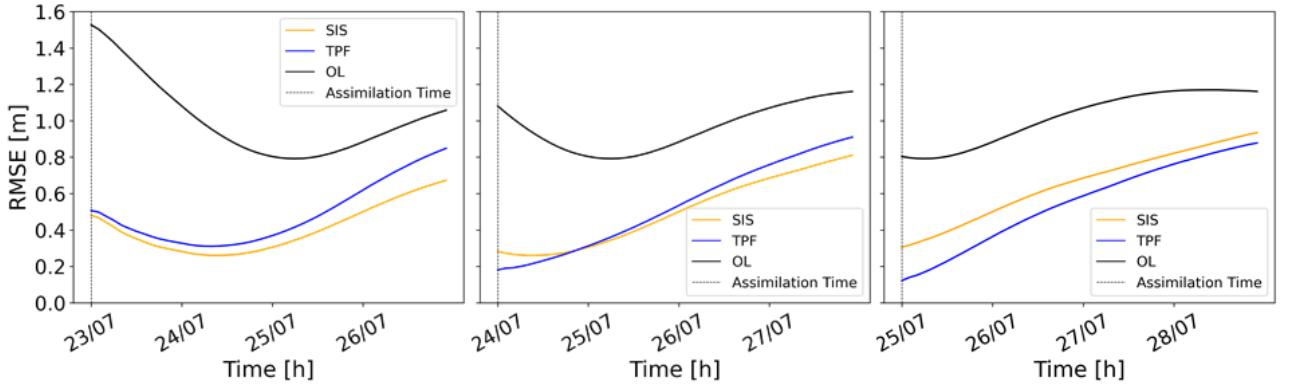
**Figure 12.** Hourly RMSE time series for a markedly biased ensemble case. The black line represents the RMSE of the OL, the blue line the RMSE after the TPF application and the orange line the RMSE after the SIS application. Assimilation at 07/23 00:00, 07/24 00:00 and 07/25 00:00 are plotted.
