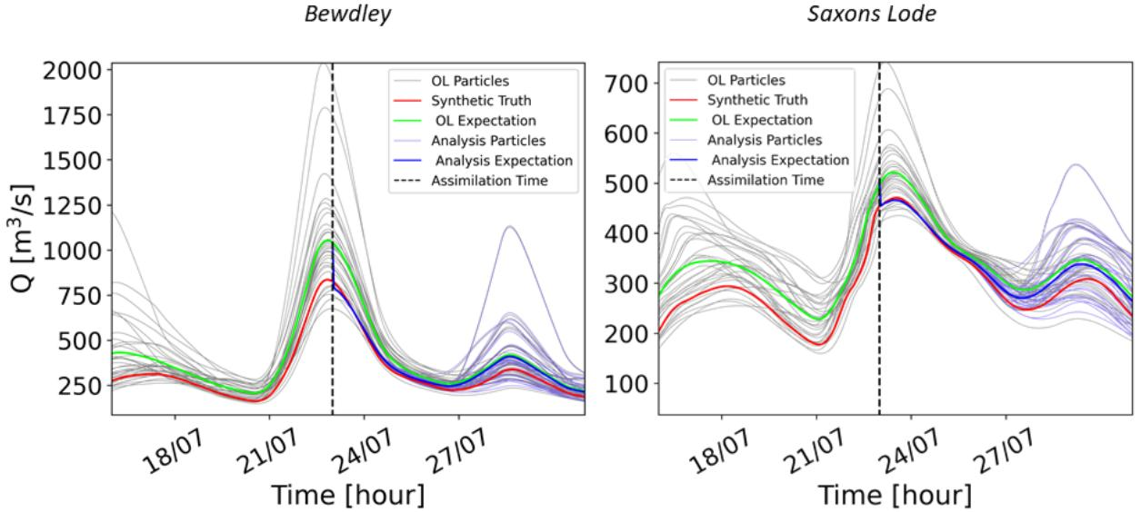
**Figure 6.** Time series of discharge at the peak at Bewdley and at Saxons Lode with the assimilation of an image at 07/23 00:00. The vertical dashed lines indicate the time of the assimilation. The gray lines correspond to the OL particles, the green line to the OL mean, the light blue lines to the analysis particles and the blue line to the analysis expectation. The synthetic truth is represented by a red line.
