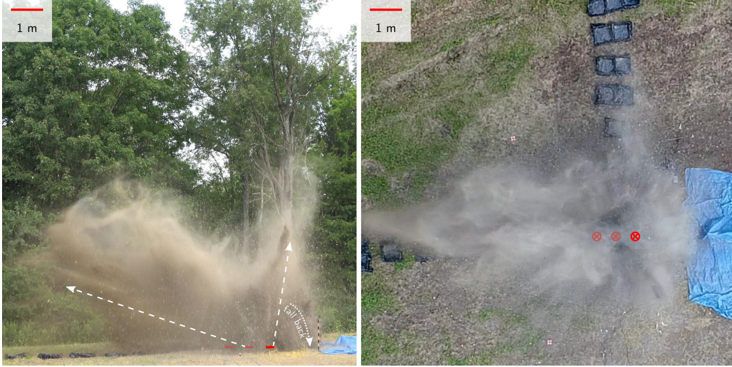
Figure 1: Side- and top view of a typical asymmetric ejecta jet created by the detonation sequences. Red markers show surface of charge locations. The example shows the jet of the third detonation in the “pad 1” configuration (See also supporting video S1).
