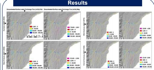
Positive values show the volume of water entering the stream from the aquifer, and the negative values indicate the volume seeps from the stream to the aquifer.
