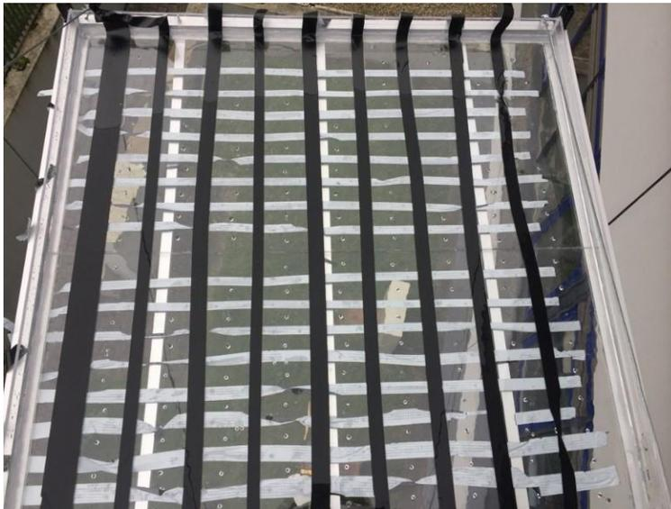
**Figure S2.** Picture of the rain generator: The outer aluminum frame (1 x 1 x 0.05 m) was filled with water and raindrops formed at regularly arranged holes in the transparent bottom plate. The rainfall rate was varied by closing or opening a varying number of holes using adhesive tape (visible as black and silver tape stripes in the picture).
