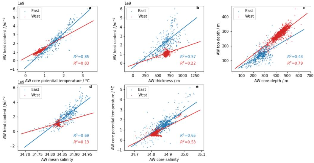
**Figure 14.** Scatter plots between (a) AW core potential temperature and total AW heat content, (b) AW layer thickness and AW heat content, (c) AW core depth and AW top depth, (d) AW mean salinity and AW heat content, and (e) AW core salinity and AW core potential temperature. Blue data is from the eastern Arctic, with red data from the western Arctic (regions defined in Figure 1). R-squared values and regression lines are shown for each scatter plot.
