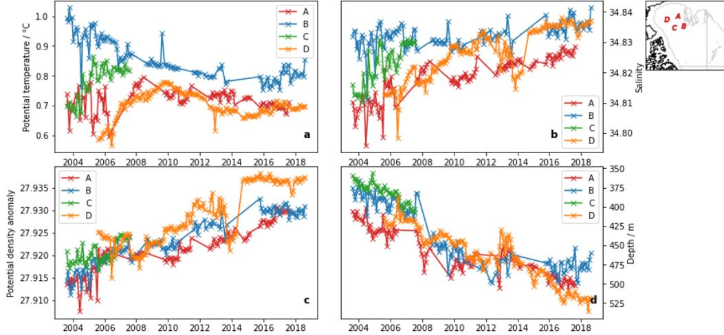
**Figure 11.** Time series of monthly mean AW core (a) potential temperature, (b) salinity, (c) potential density anomaly, and (d) depth from the four Canada Basin moorings. Mooring locations (A-D) are shown on the map at the top right.
