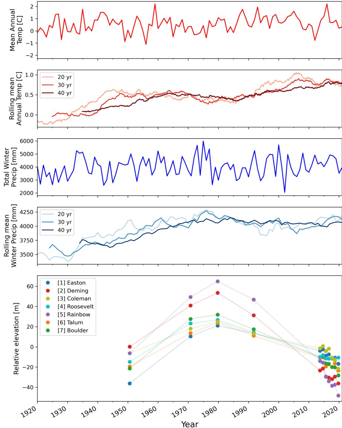
**Figure 6.** Climate and elevation change time series at Mount Baker. The relative elevation shown in the bottom panel is the elevation - mean elevation at each sample location. There appears to be a relationship between rolling mean winter precipitation values and glacier elevation change. The 40 year rolling mean Winter precipitation may present the strongest correlation, which indicates a ~40 year glacier response time.
