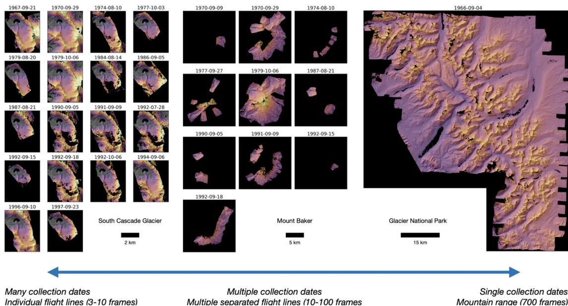
**Figure 2.** The HSfM processing pipeline derives accurate DEMs under a variety of image acquisition conditions. Image overlap is automatically detected, prior to DEM reconstruction and co-registration.
