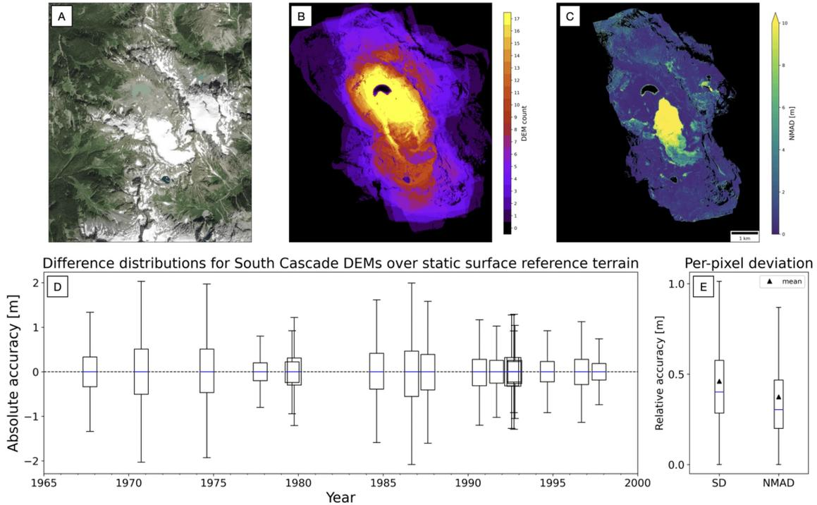
**Figure 5.** [A] South Cascade Glacier seen in 2020 Maxar basemap [9]. [B] DEM count. [C] Normalized Median Absolute Deviation (NMAD) of elevation values across all DEMs. [D] NMAD of elevation values for all DEMs over stable ground terrain, with respect to the 2013-2015 composite WV 2 m reference DEM, as a measure of absolute accuracy. [E] Standard Deviation (SD) and NMAD over stable ground terrain for all historical DEMs, as a measure of relative accuracy.
