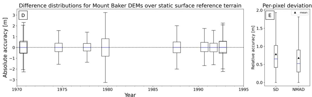
**Figure 4.** [A] Terminus locations over 2019 Maxar basemap [8]. [B] DEM count at each terminus location. [C] Normalized Median Absolute Deviation (NMAD) of elevation values across all DEMs. [D] NMAD of elevation values for all DEMs over stable ground terrain, with respect to the 2015 LiDAR 1 m reference DEM, as a measure of absolute accuracy. [E] Standard Deviation (SD) and NMAD over stable ground terrain for all historical DEMs, as a measure of relative accuracy.
