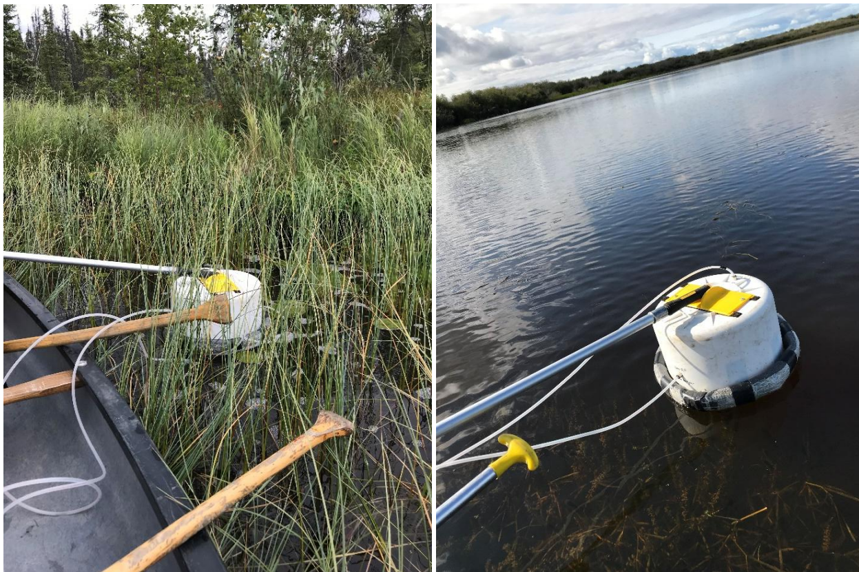
Figure S.6: Photos of emergent macrophyte (left) and open water (right) chamber flux collection.
