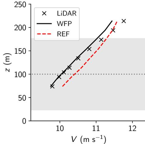
**Figure 7.** Vertical profiles of wind speed, from the reference run without wind-farm parameterisation (REF) and experiment with wind-farm parameterisation (WFP), compared to the Westermost rough lidar.
