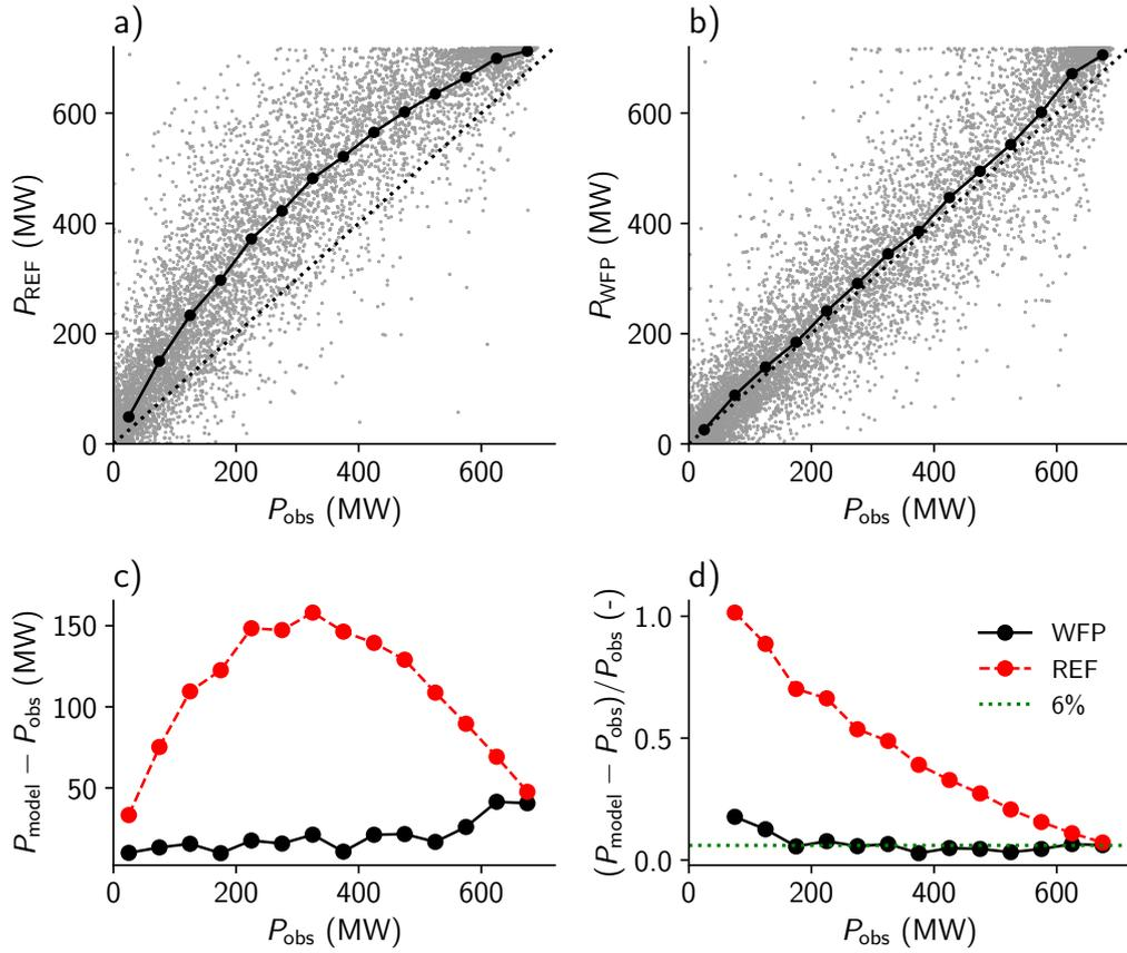
**Figure 9.** Power production calculated from the (a) reference reanalysis (REF) and (b) experiment with wind-farm parameterisation (WFP), compared to the Elia measurements. The solid black line with markers (top row) indicates the mean of the model data calculated over 50 MW bins. The bottom row shows the absolute (c) and relative (d) error of both model experiments.
