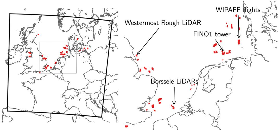
**Figure 2.** Overview of all (2.5×2.5 km) grid points with one or more wind turbines (red). Black arrows indicate the locations of measurements used for evaluation. In the left figure the black square indicates the model domain and the grey square the location of the right panel.
