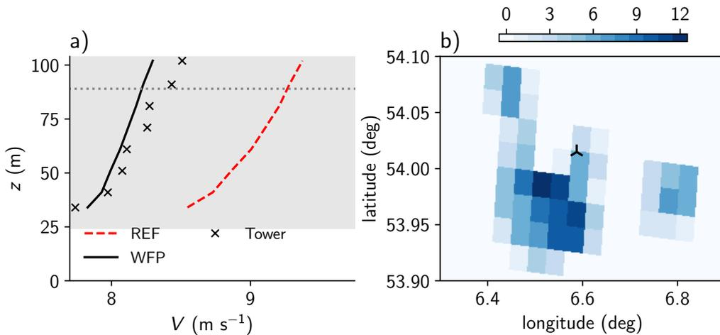
**Figure 6.** (a) Vertical profiles of wind speed, from the reference run without wind-farm parameterisation (REF) and experiment with wind-farm parameterisation (WFP), compared to the FINO1 tower. (b) The number of turbines in the HARMONIE grid cells surrounding FINO1
