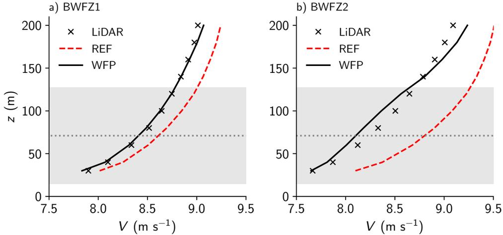
**Figure 5.** Vertical profiles of wind speed, from the reference run (REF) and experiment with wind-farm parameterisation (WFP), compared to the Borssele (a) BWFZ lidar 1, 10 km from the nearest wind farm and (b) BWFZ lidar 2, 2 km from the nearest wind farm. The grey dotted line indicates the mean hub height of the nearest wind farm and the grey shaded areas the area the diameter of the rotor.
