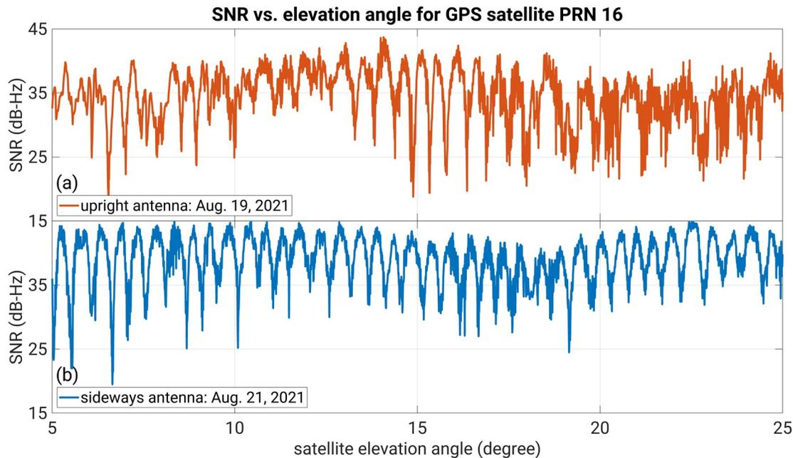
439 **Figure 6.** Examples of 1-second Signal-to-Noise Ratio (SNR) data for (a) upright and (b)
