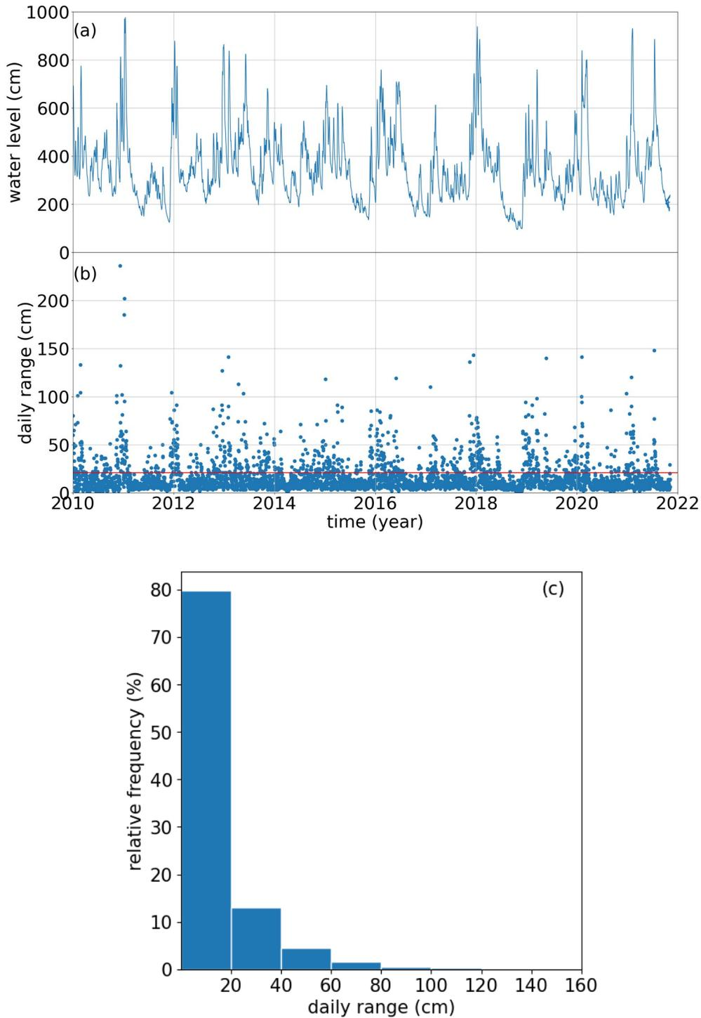
**Figure S1.** (a) 15-minutes records of river level from the river gauge at Wesel, Germany. (b) daily range values. The horizontal red line marks daily range of 20 cm. (c) relative frequency histogram for daily range data.
