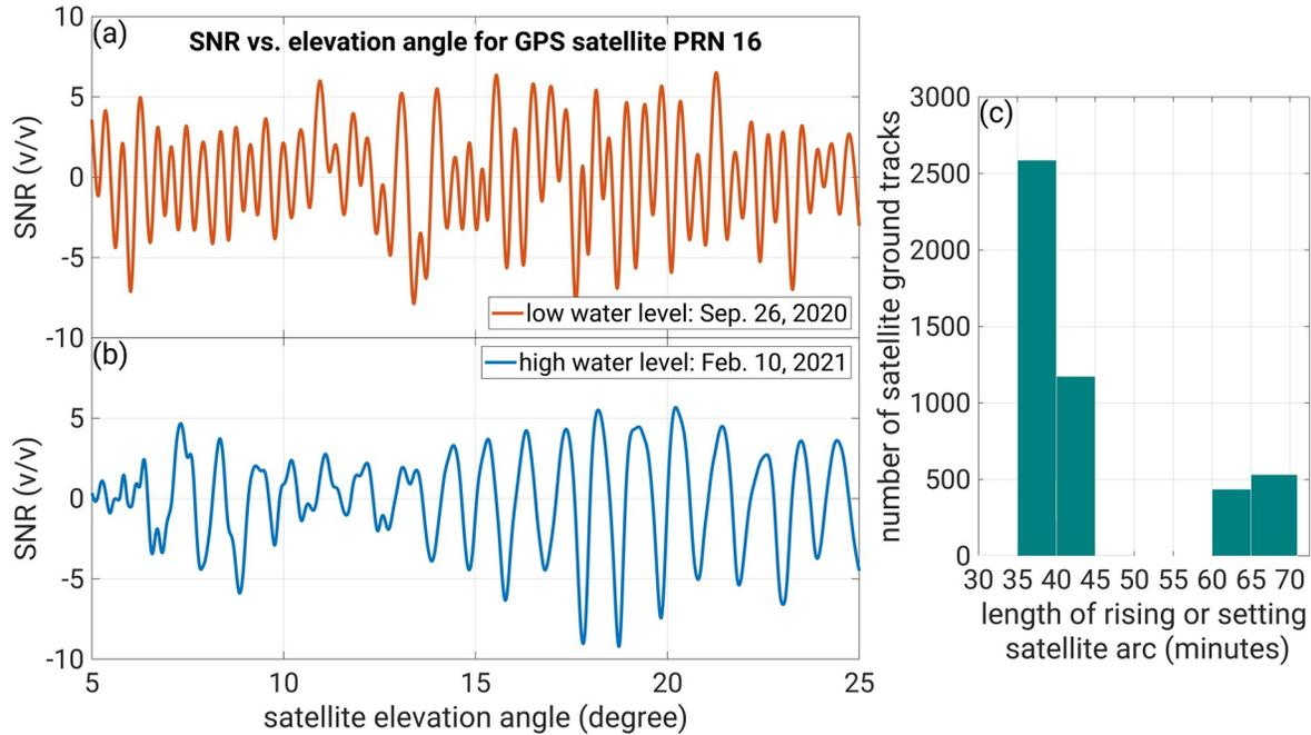
390 **Figure 4.** Detrended SNR data (after removing the direct signal) for upright RPR antenna during
