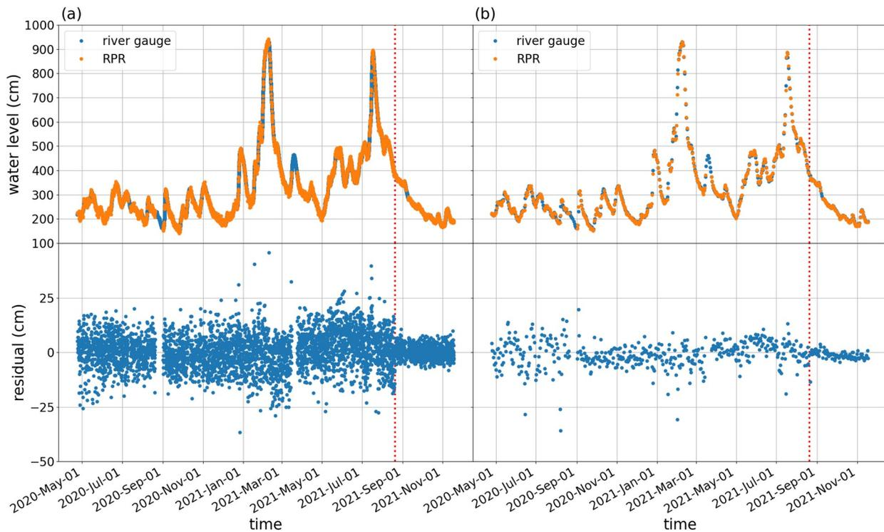
418 **Figure 5.** Water level from the river gauge and RPR. **(a)** sub-daily **(b)** daily mean. The lower
