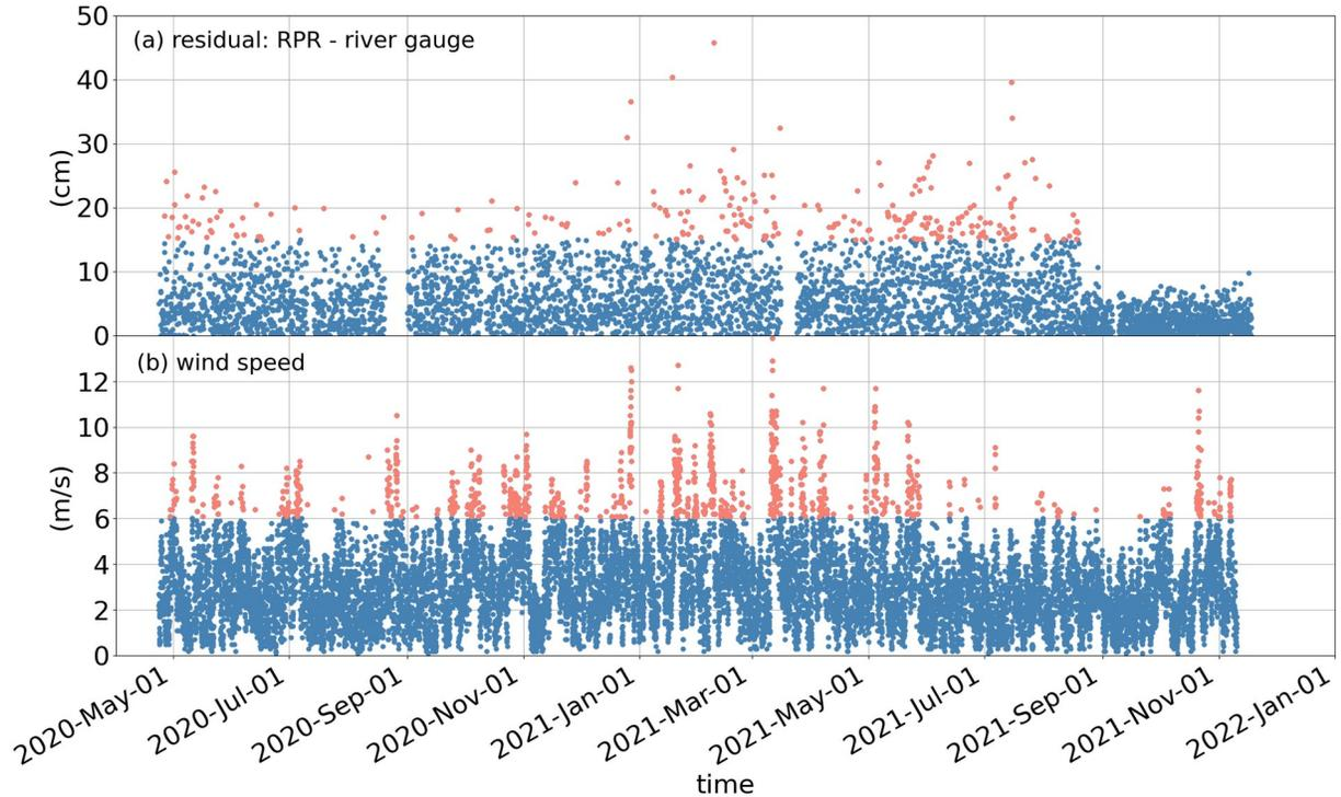
471 **Figure 7. (a)** Absolute value of water level residuals between the river gauge and RPR
