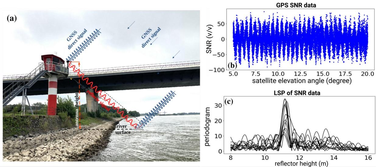
360 **Figure 3.** (a) GNSS Interferometric Reflectometry (GNSS-IR) geometry for a horizontal planar
