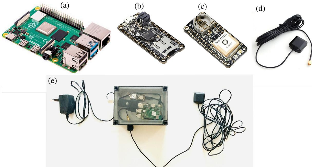
219 **Figure 1.** The RPR hardware array comprising: (a) Raspberry Pi 4 Model B (b) Adafruit Feather
