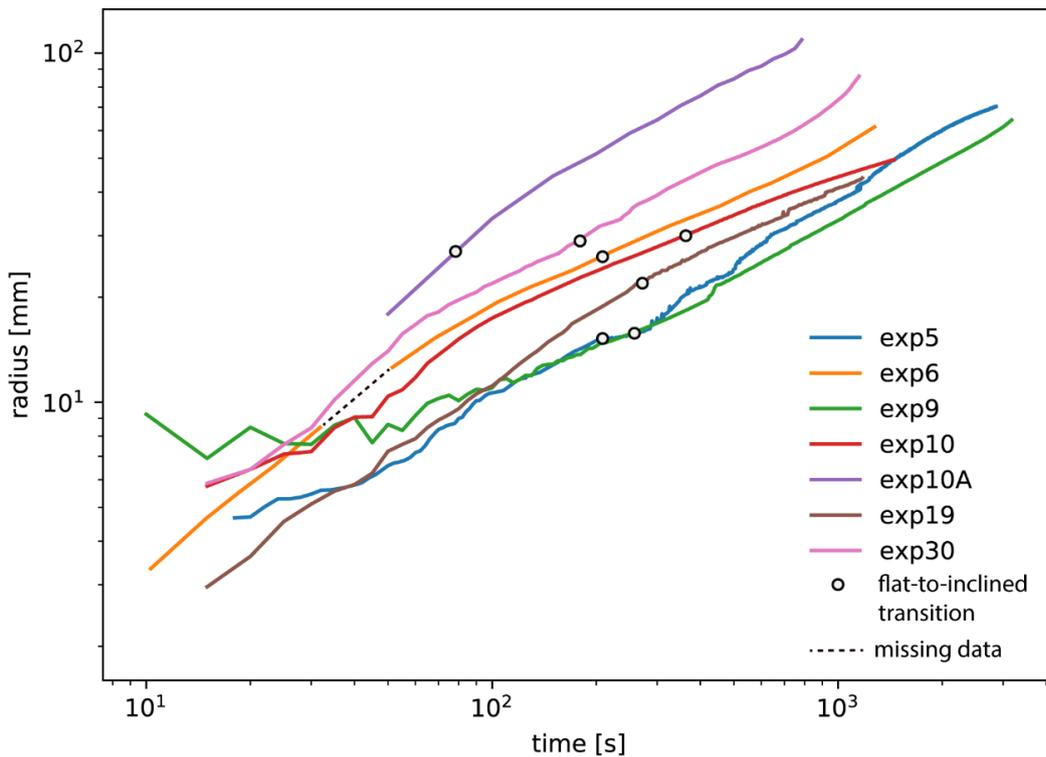
**Figure 8.** The average radius for sills in experiments (in map view) with rigidity ratio  $E_r < 4$  plotted as the best fit radius against time. The black open circles on each curve represent the transition from inner flat sill to inclined sheet of saucer-shaped intrusions. See Table 2 for the details of the experiments.
