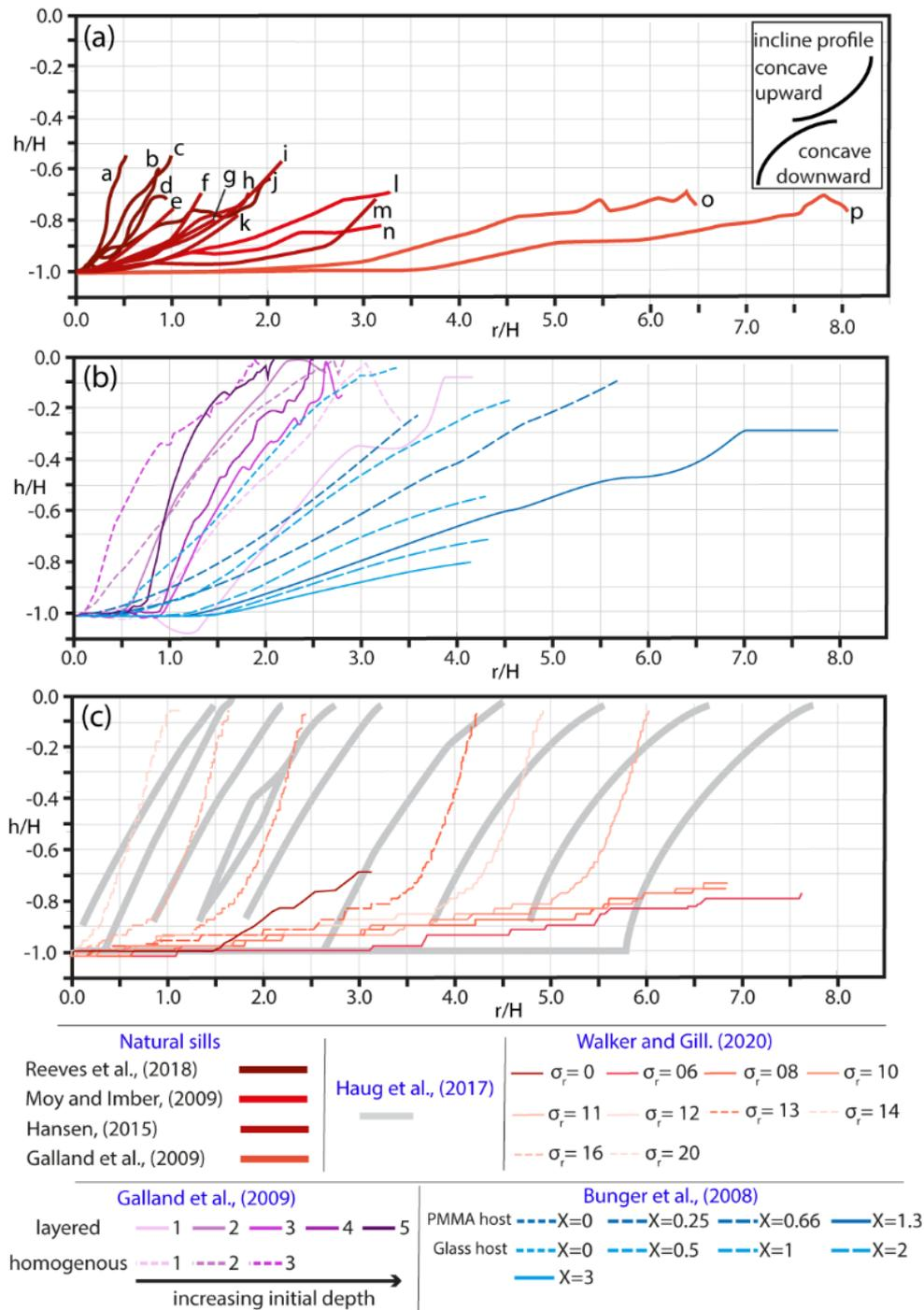
141 **Figure 2.** A comparison of saucer-shaped sill geometry in (a) nature, (b) experimental and (c)
