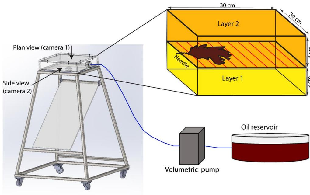
232 **Figure 3.** Schematic diagram of the experimental setup used in this study. A volumetric peristaltic pump
