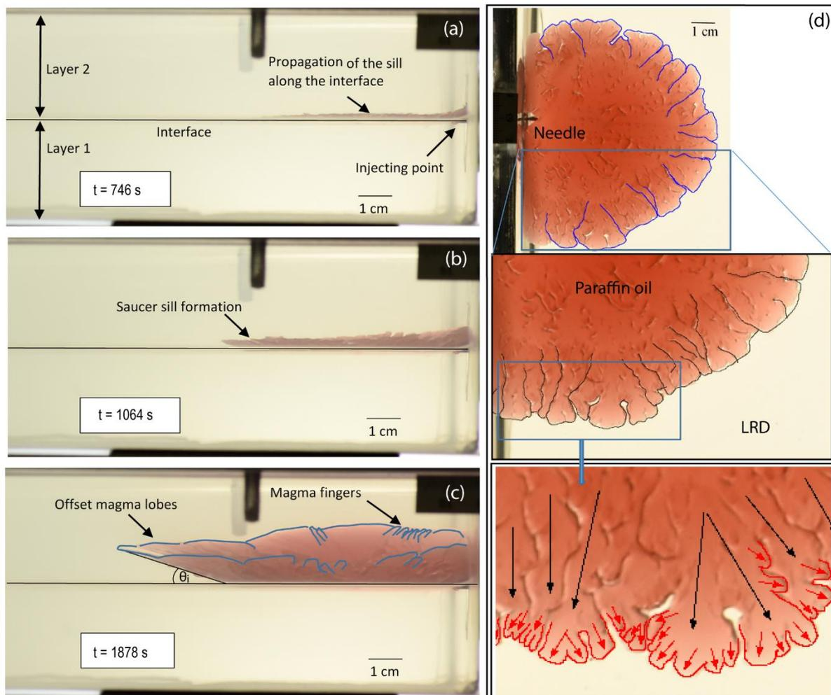
402 **Figure 5.** Side views (left panels) and top views (right panels) of sill propagation in a two-layer
