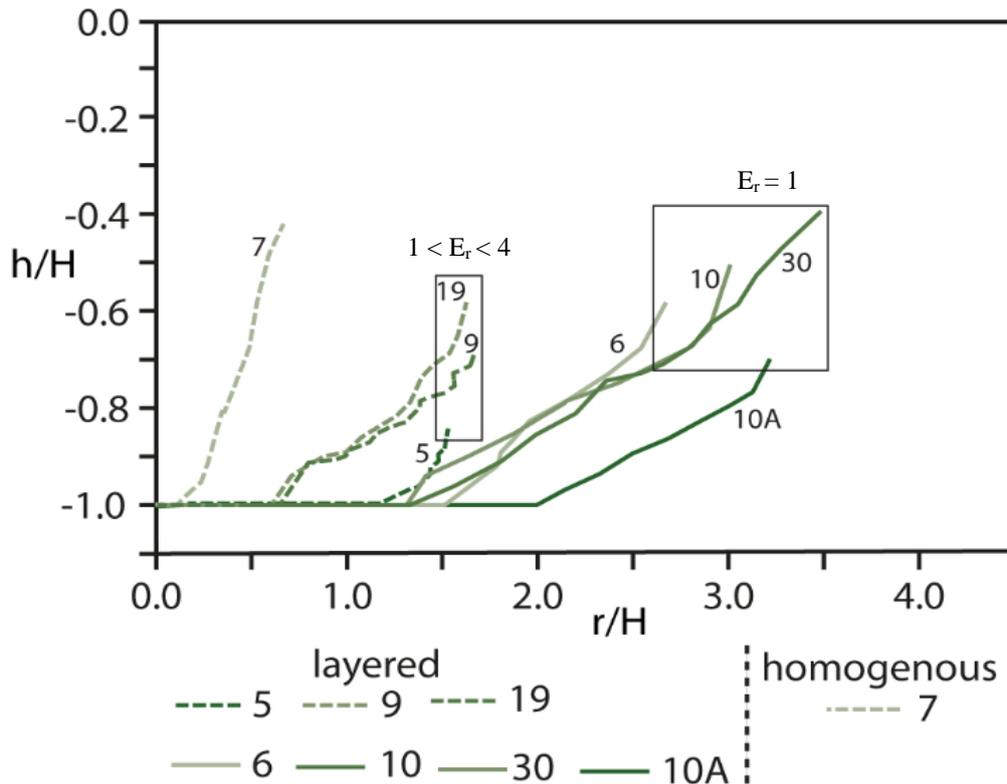
452 **Figure 6.** Normalised vertical profiles of sills observed in homogeneous and two-layer experiments.
