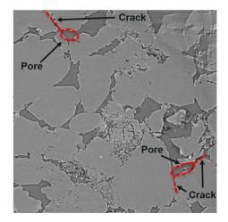
Figure 2: Raw synchrotron radiation X-ray tomographic microscopy image of dry Berea sandstone. One slice of the total data cube with  $1024^3$  voxels [from Madonna et al. (2013)]. Alkhimenkov Y. and Quintal B. –
