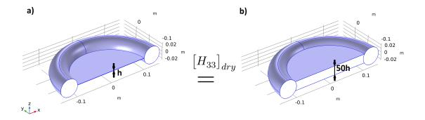
Figure 17: Sketch illustrating the pore space (dry) of the Big pore model with two different crack apertures — h (left) and 50h (right). Alkhimenkov Y. and Quintal B. –
