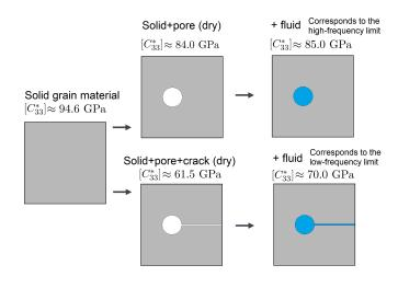
Figure 6: Sketch illustrating the configurations of our model that corresponds to the highand low-frequency limits obtained from the numerical calculations for the  $[C_{33}^*]_{sat}$  component (properties in Tables 1 and 2).
