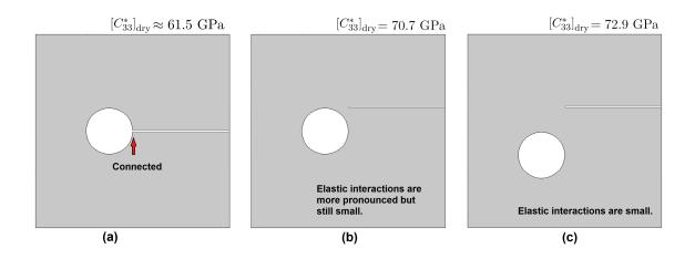
Figure 16: A slice of the three-dimensional models illustrating the effect of elastic interactions on the  $[C_{33}^*]_{dry}$  component. (a) The isometric pore is connected to the crack representing a unified interconnected pore space, (b) the isometric pore and crack are disconnected but close and (c) disconnected and far from each other. **Alkhimenkov Y. and Quintal B.** –
