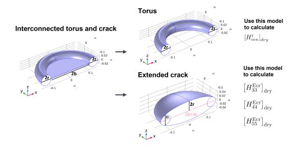
Figure 7: Sketch illustrating the workflow for calculating analytically different components of the compliance matrix for the model with interconnected isometric pore and crack. Alkhimenkov Y. and Quintal B. –
