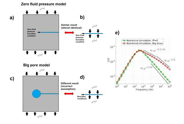
Figure 8: Sketch illustrating the simplifications made in analytical models via applied boundary conditions (a vertical slice of the two models shown in Figure 4). Panels a) and c) — boundary conditions applied to the walls of the model. Panels b) and d) — boundary conditions applied to the walls of the crack. Panel e) shows the numerical result; note, that the high-frequency slope of the attenuation curve is substantially different if the crack is connected to an actual pore.
