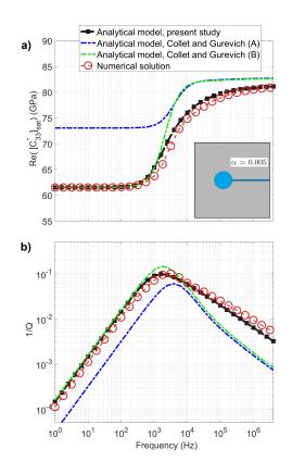
Figure 13: Numerical and analytical results for the Big pore model with the crack aspect ratio  $\alpha = 0.005$  (i.e., finite thickness crack): (a) Real part of the  $[C_{33}^*]_{\text{sat}}$  component and (b) dimensionless attenuation for the  $[C_{33}^*]_{\text{sat}}$  component. Here the crack aperture is two times larger than in the model with aspect ratio of  $\alpha = 0.0025$  (Figure 12). The inset represents the cross section of half of the model.
