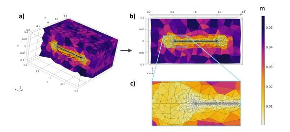
Figure A-1: The element's size distribution for the Big pore model. The element's size in the crack is  $\approx 6 \times 10^{-4}$  m, and in the surrounding grain material it is  $7.2 \times 10^{-3} - 4 \times 10^{-2}$  m. The element's size distribution for the other models is similar. The total number of elements is  $1.5 \times 10^6 - 5 \times 10^6$  depending on the model configuration, e.g., Big/Small pore or full/half/quarter of a model was used.
