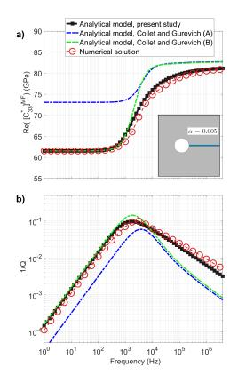
Figure 14: Numerical and analytical results for the modified frame of the Big pore model with the crack aspect ratio  $\alpha = 0.005$  (i.e., finite thickness crack): (a) Real part of the  $[C_{33}^*]^{\rm MF}$  component and (b) dimensionless attenuation for the  $[C_{33}^*]^{\rm MF}$  component. The inset represents the cross section of half of the model.
