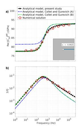
Figure 15: Numerical and analytical results for the modified frame of the Small pore model with the crack aspect ratio  $\alpha = 0.0025$ : (a) Real part of the  $[C_{33}^*]^{\text{MF}}$  component and (b) dimensionless attenuation for the  $[C_{33}^*]^{\text{MF}}$  component. The inset represents the cross section of half of the model.
