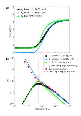
Figure 11: The real part of the frequency-dependent fluid bulk modulus  $K_f^*$  and the dimensionless attenuation calculated using different expressions for the Small pore model with  $\alpha = 0.0025$ .
