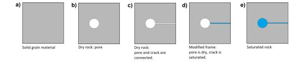
Figure 5: Cartoon illustrating the different model configurations used to obtain the corresponding compliance matrices.
