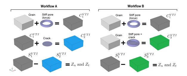
Figure B-1: Sketch illustrating the calculation of normal and tangential compliances of the crack for workflows A and B.  $S_r^{VTI}$  denotes the compliance tensor, which is the inverse of the corresponding stiffness tensor, i.e.,  $S_r^{VTI} = (C_r^{VTI})^{-1}$ , for r = 1, 2, 3. The resulting  $Z_n$  and  $Z_t$  are used to calculate the analytical solution for corresponding models. Alkhimenkov Y. and Quintal B. –
