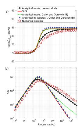
Figure 18: Numerical and analytical results for the big pore model with the crack aspect ratio  $\alpha = 0.025$ : (a) Real part of the  $[C_{33}^*]_{sat}$  component and (b) dimensionless attenuation for the  $[C_{33}^*]_{sat}$  component.
