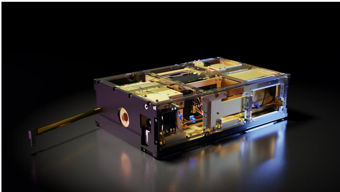
**Figure 15.** The GenSat-1 CubeSat showing AGILE payload’s circular aperture on the front face. GenSat-1 will be in high inclination LEO with AGILE looking zenith-wards over the Earth’s polar regions
