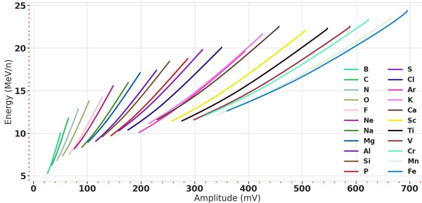
**Figure 14.** Estimated energy as a function of measured Maximum amplitude in layer 1 when the identification of particle ID is possible (Gautier et al., 2021).
