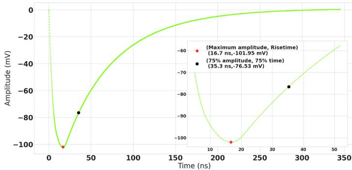
**Figure 3.** Simulated signal in the stopping layer of a stack of three Si detectors, each 300 microns thick. In this instance, the signal is produced by a 20 MeV/n Oxygen ion stopping in the second layer. The inset shows a zoomed-in view with the legend stating the numerical values of rise time and amplitude values.
