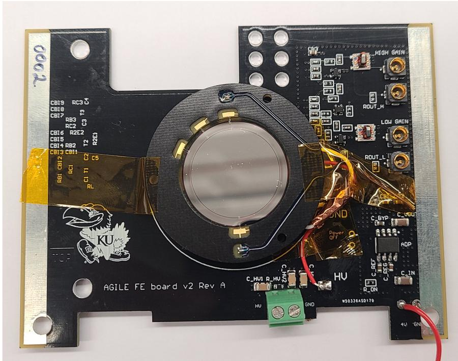
**Figure 11.** A photo of the assembled FEE board together with a SSD.
