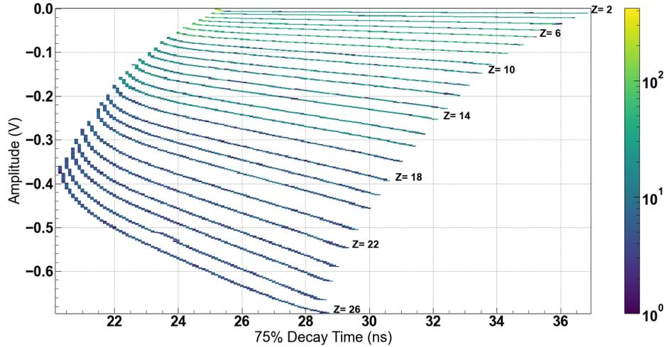
**Figure 4.** He to Fe ( $Z=2$  to 26) tracks of maximum amplitude vs rise time in the stopping layer. The tracks are well separated for each species over the full simulated energy range (3-6 MeV for He and 12-22 MeV/n for Fe) of the incident ion. Color bar to the right shows the number of particles in each energy bin. Particle ID is obtained from its characteristic track, and its energy from the amplitude (Gautier et al., 2021).
