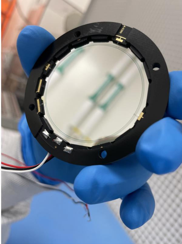
**Figure 8.** A photo of one AGILE SSD showing the packaging and the active (black), ohmic(red) and the guard ring (white) connections. Clockwise from the bottom left white/black/red wires, the Field Plate and the Multi Guard Ring and the active are connections are shown. All connections are triple bonded for redundancy.
