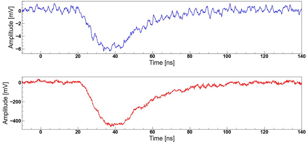
**Figure 10.** Voltage output from the FFE amplifier as a function of time in response to an alpha particle. Top panel shows the low gain and bottom panel shows high gain raw output.
