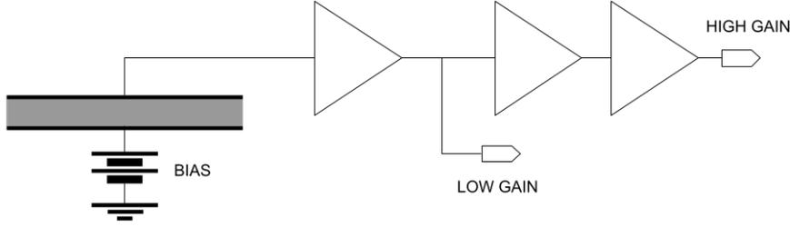
**Figure 9.** Block diagram of the triple stage amplifier. The FEE is designed to work with PSEC4 sampler ASIC. Therefore, the two output signals are always below 1V and at least one of the two will have a signal of 10 mV for the particles with very low ionization.
