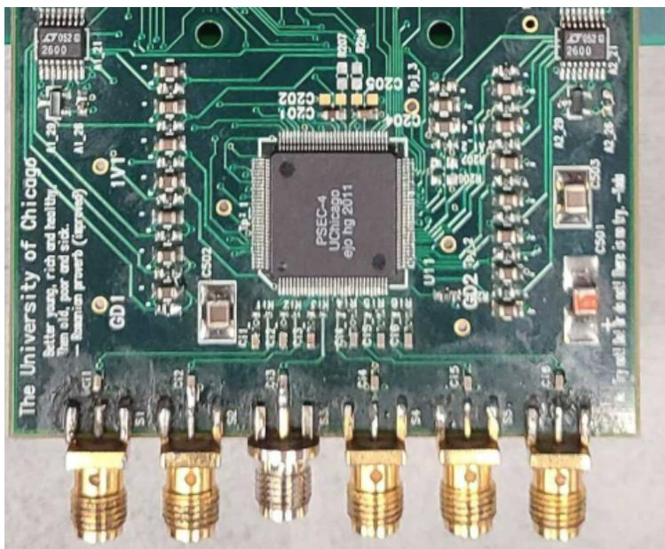
**Figure 12.** Photograph of a PSEC4 test board. The PSEC4 chip can be seen at the center of the board.
