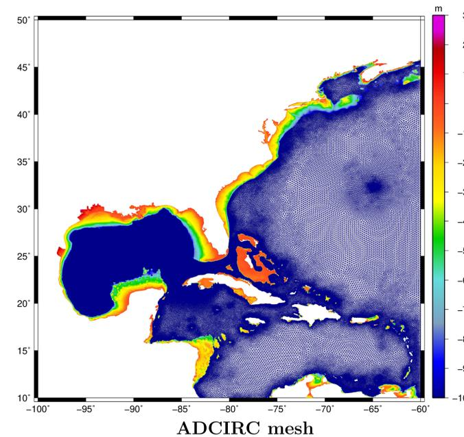
The one mesh that represents the current layout of the Ship Channel has depths of 14.33m while the mesh with the proposed dredging in the channel has a depth of 21.33m. The winds and pressure were obtained from the North American Mesoscale model (NAM), and the tidal forcing input was taken from the TPXO9 model.
