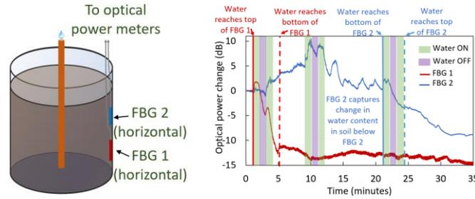
Figure 4: (a) Experimental setup for monitoring underground water level. (b) The measured optical power change against the change in water level.
