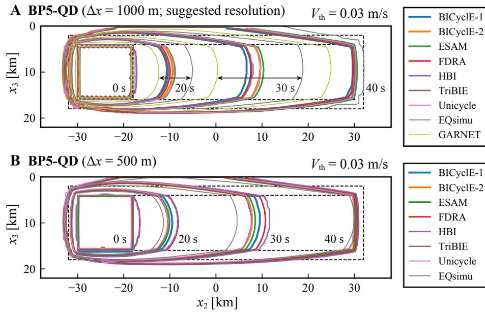
**Figure 7.** Rupture fronts of the first earthquake in BP5-QD simulations with different numerical resolutions. The contours of rupture fronts indicate 0, 20, 30, and 40 s after the earthquake initiation time in simulations with (a)  $\Delta x = 1000$  m and (b)  $\Delta x = 500$  m. The threshold slip rate for the coseismic phase,  $V_{th} = 0.03$  m/s, is different from that in Figure 4.
