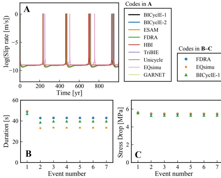
**Figure 9.** Long-term fault behavior and earthquake characteristics in BP5-QD simulations. (a) Time evolution of maximum slip rates in the seismogenic zone and (b) rupture duration and (c) stress drop for the first seven earthquakes are shown for simulations with  $\Delta x = 1000$  m.
