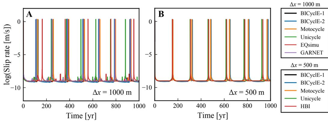
**Figure 5.** Time evolution of maximum slip rates in BP4-QD simulations. The time series of logarithmic maximum slip rates within the seismogenic zone are shown for simulations with (a)  $\Delta x = 1000$  m and (b)  $\Delta x = 500$  m. We use logarithms with base 10 and code names in legends in this and all later figures.
