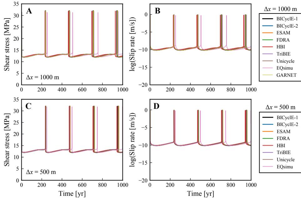
**Figure 10.** Long-term fault behavior at the surface in BP5-QD simulations. (a and c) Shear stress and (b and d) slip rates on the fault at the surface ( $x_1 = x_2 = x_3 = 0$  km) in simulations with (a and b)  $\Delta x = 1000$  m and (c and d)  $\Delta x = 500$  m.
