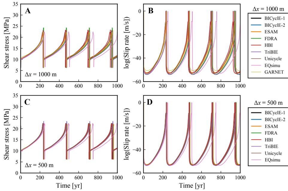
**Figure 11.** Long-term fault behavior at a seismogenic depth in BP5-QD simulations. (a and c) Shear stress and (b and d) slip rates on the fault at the mid-seismogenic depth ( $x_1 = x_2 = 0$  km;  $x_3 = 10$  km) in simulations with (a and b)  $\Delta x = 1000$  m and (c and d)  $\Delta x = 500$  m. Note that the range of vertical axes in panels b and d are different from those in Fig. 10.
