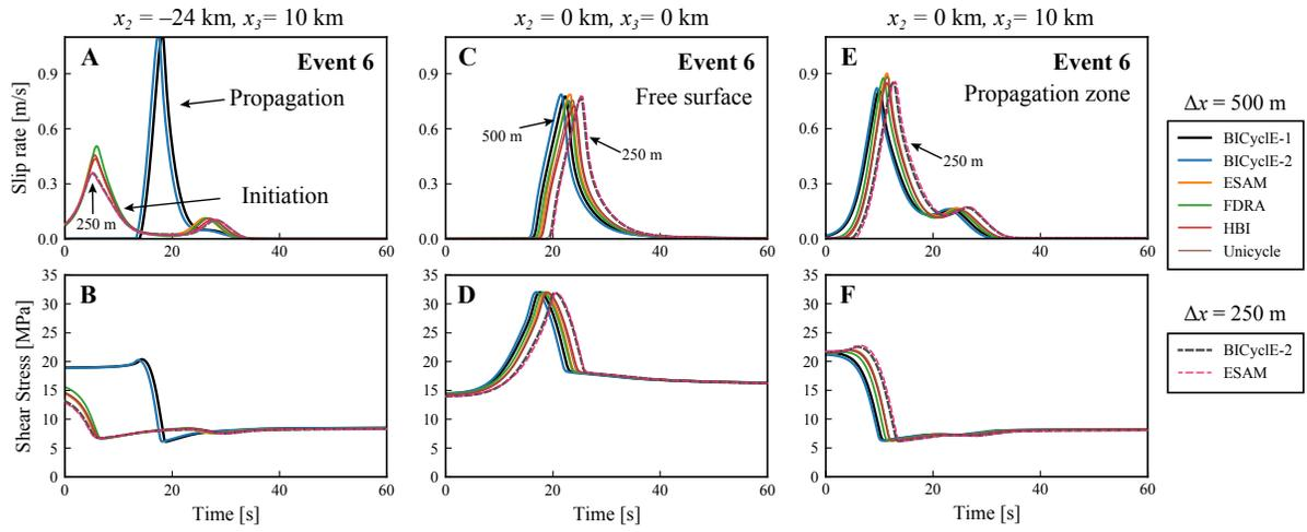
**Figure 14.** Coseismic rupture of the sixth event in BP5-QD simulations ( $\Delta x = 500$  and  $250$  m). Time evolution of (a, c, and e) coseismic slip rates and (b, d and f) shear stresses are shown at the same locations on the fault as in Figure 12. We mark the distinct signals indicating the rupture initiation or propagation for 500-m simulations, as well as the matching 250-m simulations.
