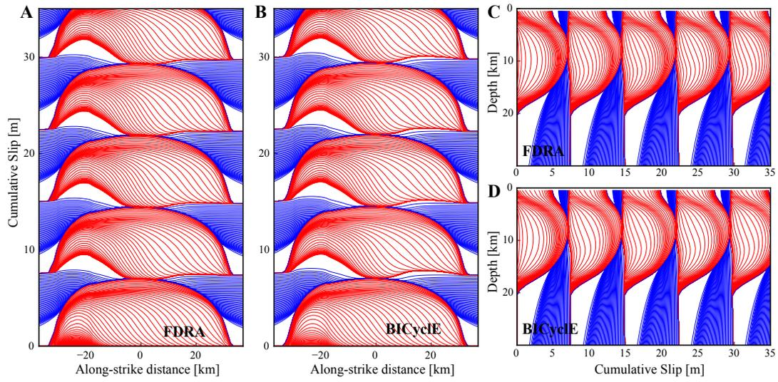
**Figure 8.** Fault slip evolution in selected BP5-QD simulations. Cumulative fault slip in two simulations ( $\Delta x = 1000$  m) using FDRA and BICycleE is plotted along (a and b) horizontal ( $x_3 = 10$  km) and (c and d) vertical ( $x_2 = 0$  km) profiles shown in Figure 3. The seismic slip (red lines) is plotted every 1 s and aseismic slip (blue lines) is plotted every 5 yr, with the threshold slip rate  $V_{th} = 0.01$  m/s.
