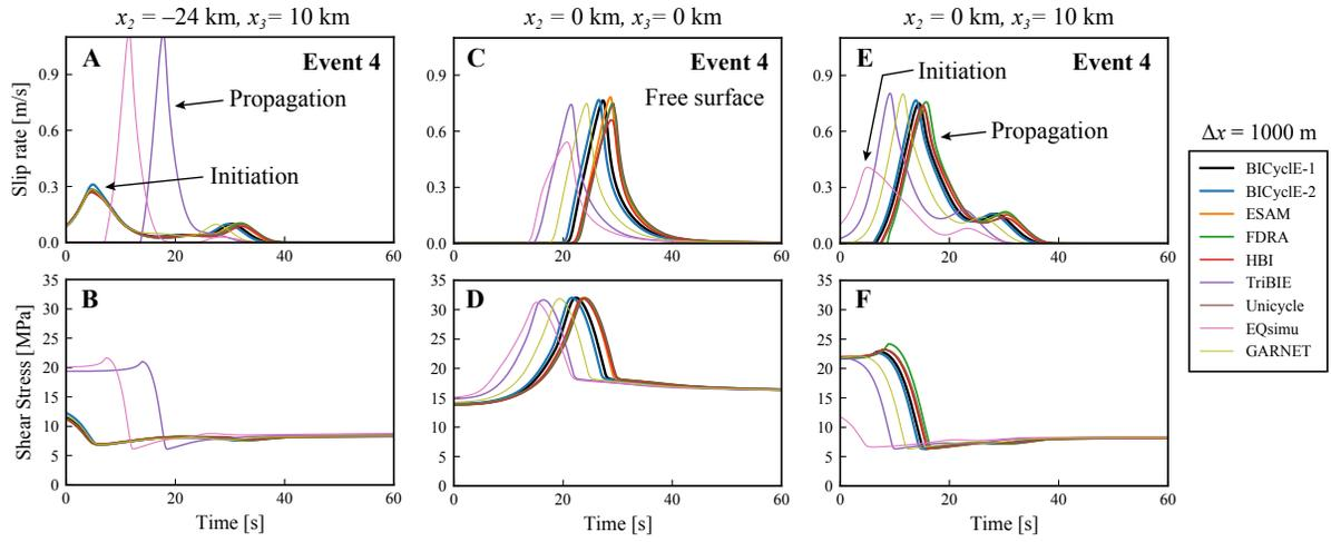
**Figure 13.** Coseismic rupture of the fourth event in BP5-QD simulations ( $\Delta x = 1000$  m). Time evolution of (a, c, and e) coseismic slip rates and (b, d and f) shear stresses are shown at the same locations on the fault as in Figure 12. The discrepancy of TriBIE and EQsimu simulations with others are due to different rupture directions. We mark the distinct signals indicating the rupture initiation or propagation in panels a and e.
