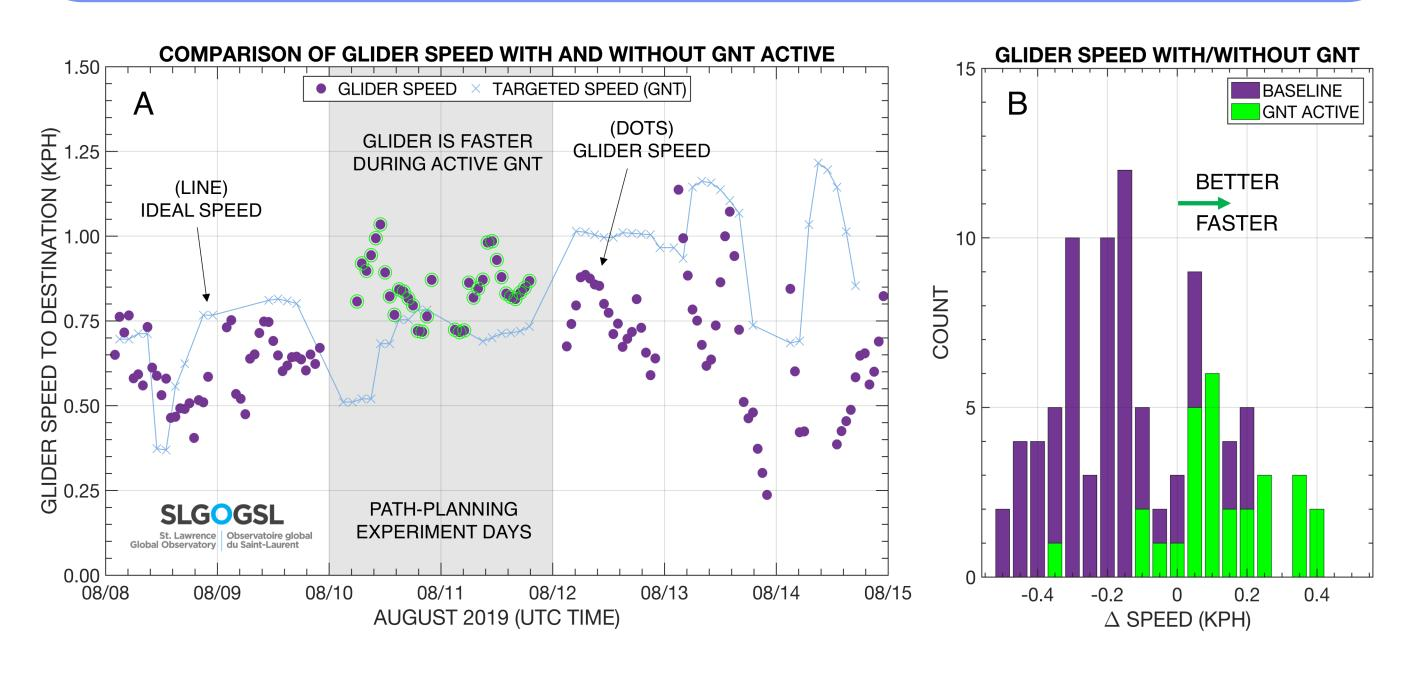
**Panel A:** Glider and GNT planned speed towards direction of destination; greyed out area highlights the path planning experiment days August 10 – 12, 2019 during which the results of the GNT were actively sent to the glider. Panel B: Difference in glider and GNT speeds showing clear improvement during active path-planning days.
