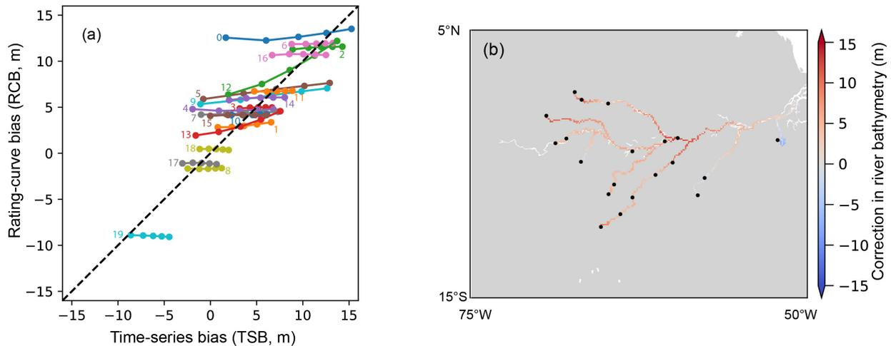
**Figure 5 (a)** Comparison of the TSB- and RCB-based river bathymetry correction methods with noise-corrupted runoff. Five dots represent results based on five runoff inputs (left to right,  $-50\%$ ,  $-25\%$ , baseline,  $+25\%$ , and  $+50\%$ ). **(b)** A sample of correction for baseline runoff using the RC-Method.
