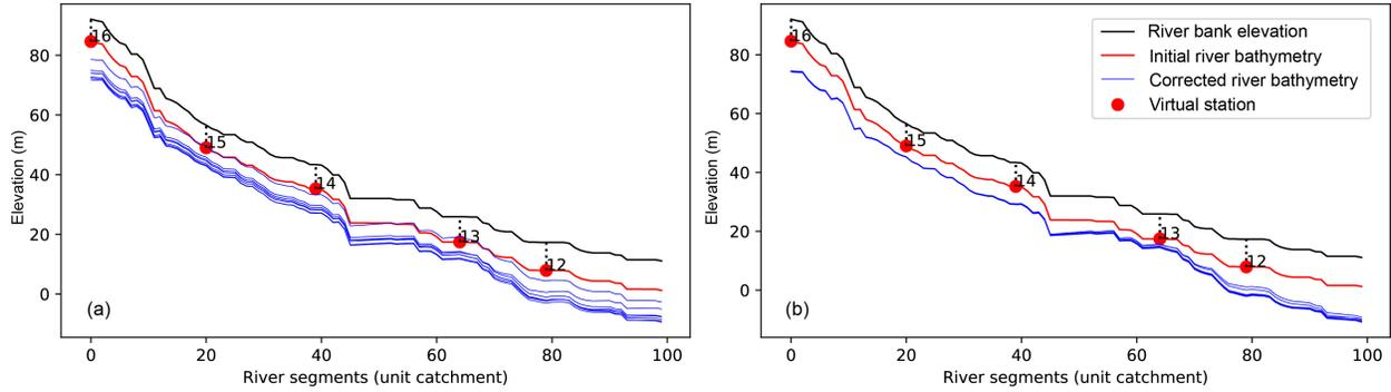
**Figure 8.** (a) and (b) illustrate the riverbank elevation, initial river bathymetry and the corrected river bathymetry with different runoff inputs using TS-Method and RC-Method, respectively. Seven different runoffs are from earth2observe project.
