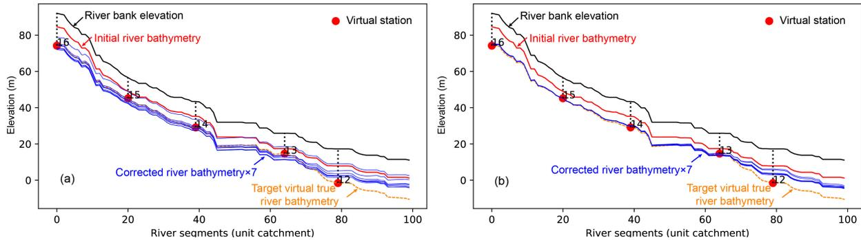
**Figure 10** Results of Observing System Simulation Experiments (OSSEs) experiment. (a) and (b) illustrate the riverbank elevation, initial river bathymetry and the corrected river bathymetry with seven different earth2observe runoff inputs using TS-Method and RC-Method, respectively. We assumed the “virtual true” target river bathymetry (orange lines). The efficiency of correction will be compared with the target river bathymetry.
