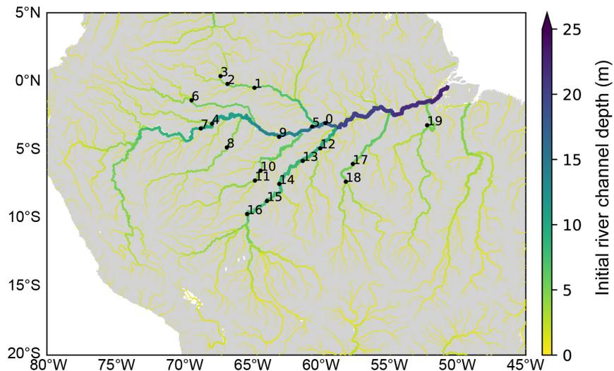
**Figure 3** The location of the selected virtual stations in the Amazon River Basin. The Initial River channel depths was approximated using the empirical power law equation (Eq. 1). River segments with depths of  $< 2.5 \text{ m}$  were filtered out.
