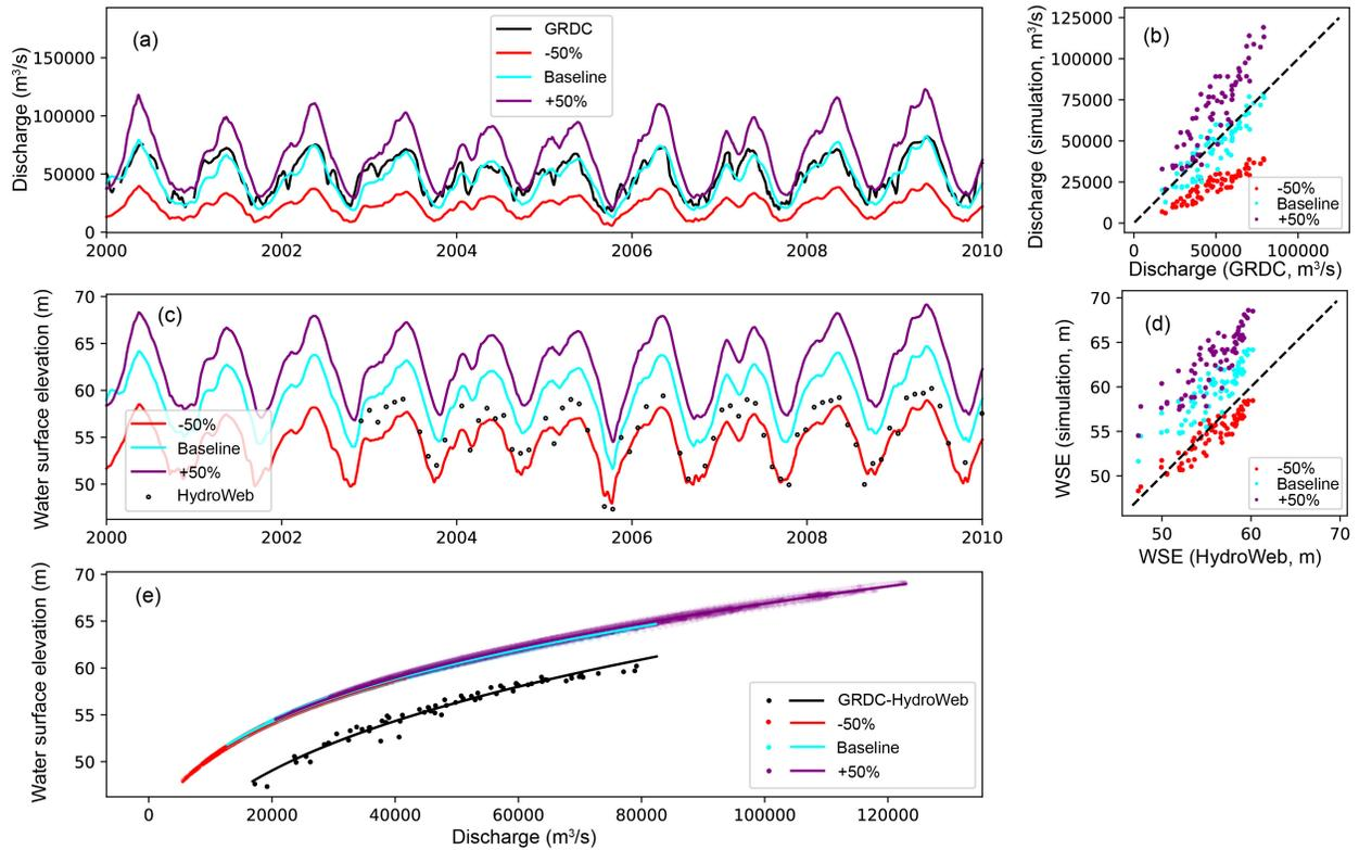
**Figure 4** Comparison of model simulations and observations for (a, b) time series river discharge data, (c, d) WSE, and (e) rating curves for gauge 7 (San Paulo De Olivenca, Amazon River). Solid lines in (e) are the rating curves fitted to observations (color) and simulations (black).
