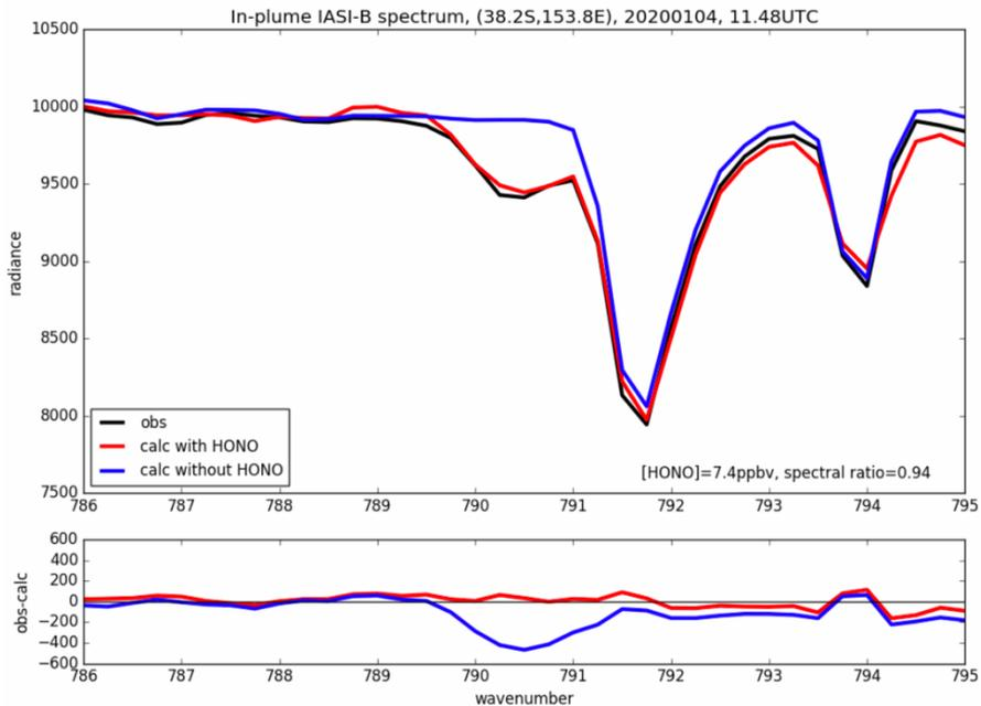
**Figure S1.** Example of a spectrum measured within an Australian fire plume detected on 4 January 2020 at 11.48 UTC by IASI-B. The observed spectrum (black) is compared to the direct radiative transfer calculation with (red) and without (blue) HONO included. The difference between the observed and the calculated spectra is displayed in the lower panel. The HONO contribution is visible between 790 and 791  $\text{cm}^{-1}$ .
