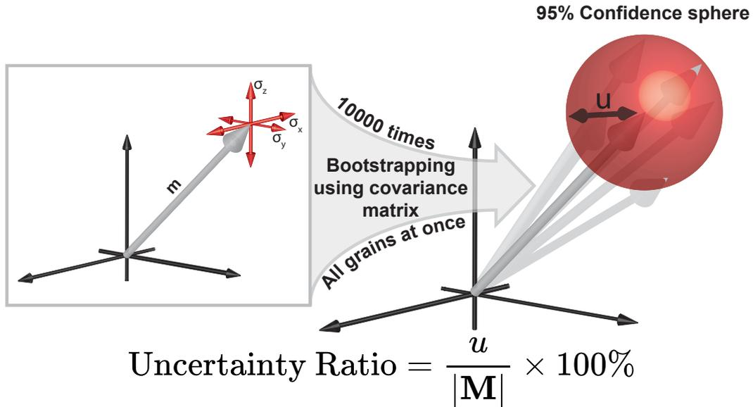
**Figure 2.** The construction of the uncertainty ratio. The covariance matrix is bootstrapped to generate a set of 10,000 possible magnetization vectors around mean magnetization vector  $\mathbf{M}$ . The radius of a sphere containing 9,500 of the end-points of these vectors is defined as the 95% confidence sphere with radius  $u$ . The length of the magnetization vector  $|\mathbf{M}|$  and  $u$  are then used to define the uncertainty ratio of a solution.
