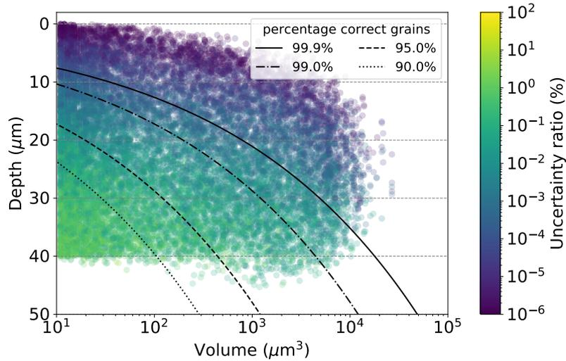
**Figure 6.** Using the SSR to select subsets of grains with accurately resolved magnetizations for our models with a grain density of  $10^5$  grains per  $\text{mm}^3$ , sampling interval of  $1 \mu\text{m}$ , and noise level of  $5 \text{ nT}$  for a  $500 \times 500 \times 50 \mu\text{m}$  sample surface. The grains are colored according to their uncertainty ratio. Four different SSRs select 99.9, 99.0, 95.0, and 90.0% of the grains with an uncertainty ratio of maximum 10%.
