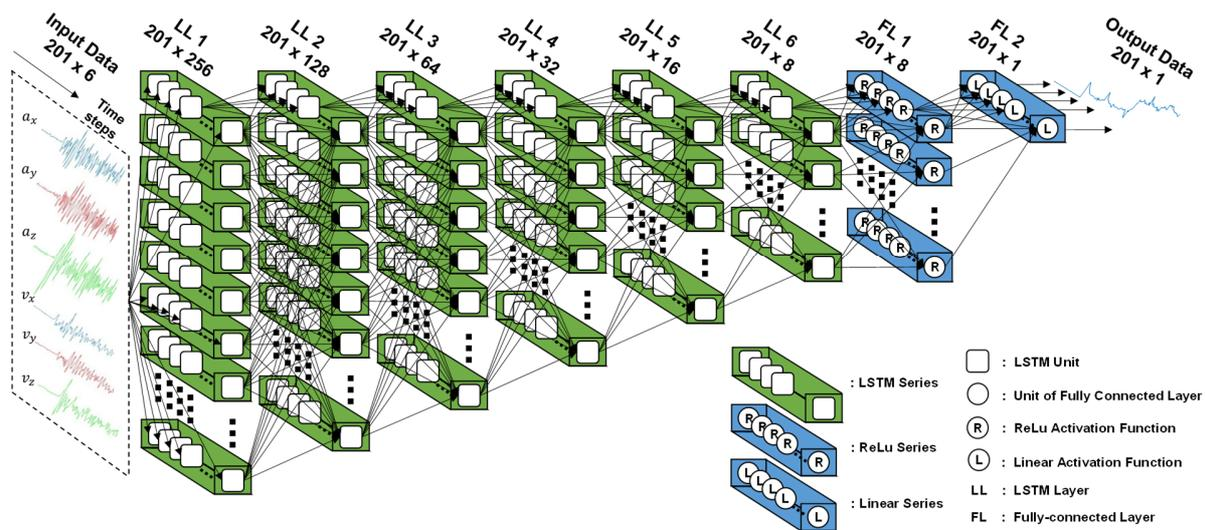
**Figure 4.** Proposed architecture of the LSTM model.
