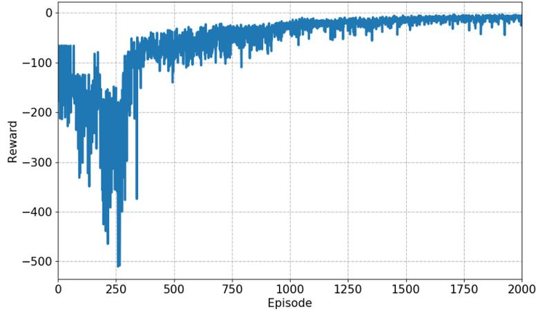
**Figure 10.** Reward history received by the RL agent when using reward function 2. The reinforcement-learning-based control is achieved in less than 500 learning episodes. The entire training process of 2000 episodes takes 122 seconds on an Intel® Xeon® E5-1650 v3 CPU. Notably, the reward improves with the increase in learning episodes.
