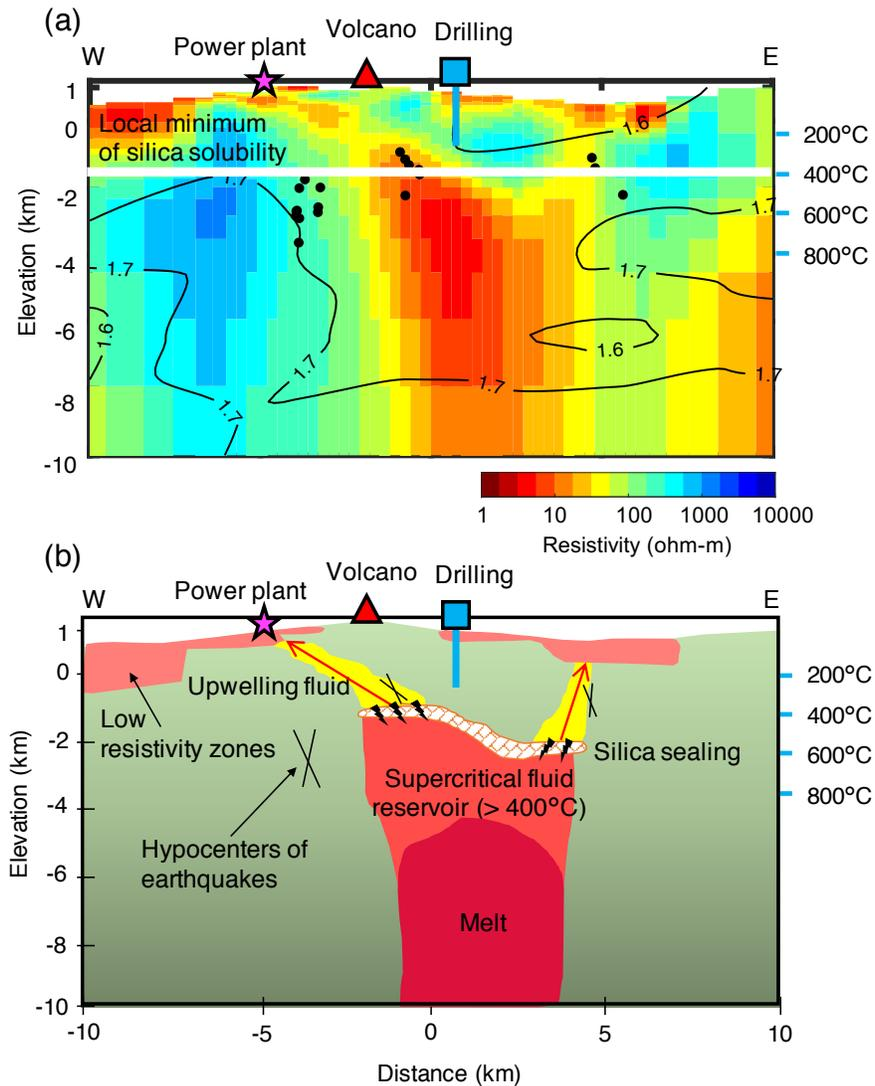
504 **Figure 9.** (a) West–east cross-section at  $x = 0.5$  km of the inverted resistivity model. This cross-
