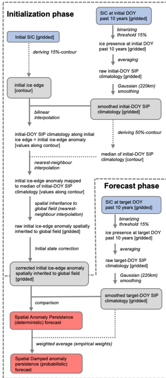
**Figure S1.** Schematic of the Spatial Damped Anomaly Persistence method as described in the main publication. The only data used as input for the method is SIC at initial date and climatological SIC, found using the SIC for the same DOY for the past 10 years. Further information is in the main text.
