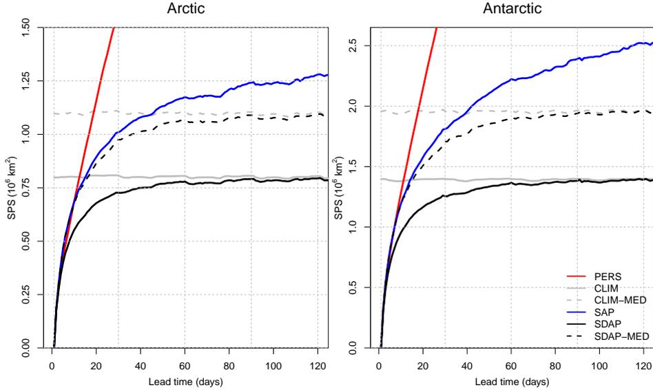
**Figure 2.** Spatial Probability Score (SPS) at increasing lead times (in days) for all forecasts averaged across all forecasts initialised between 1999 and 2020. The two dotted lines (CLIM-MED and SDAP-MED) are binary forecasts derived by assigning the ice edge at the 50% contour of the probabilistic forecasts (CLIM and SDAP). Further details are in the text.
