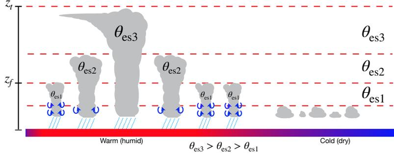
**Figure 2.** A schematic of tropical convection and temperature. Colors at the surface represents the sea surface temperature. Blue arrows represent the entrainment process. The height of the convective top is denoted by  $z_t$ . The freezing level is denoted by  $z_f$ .
