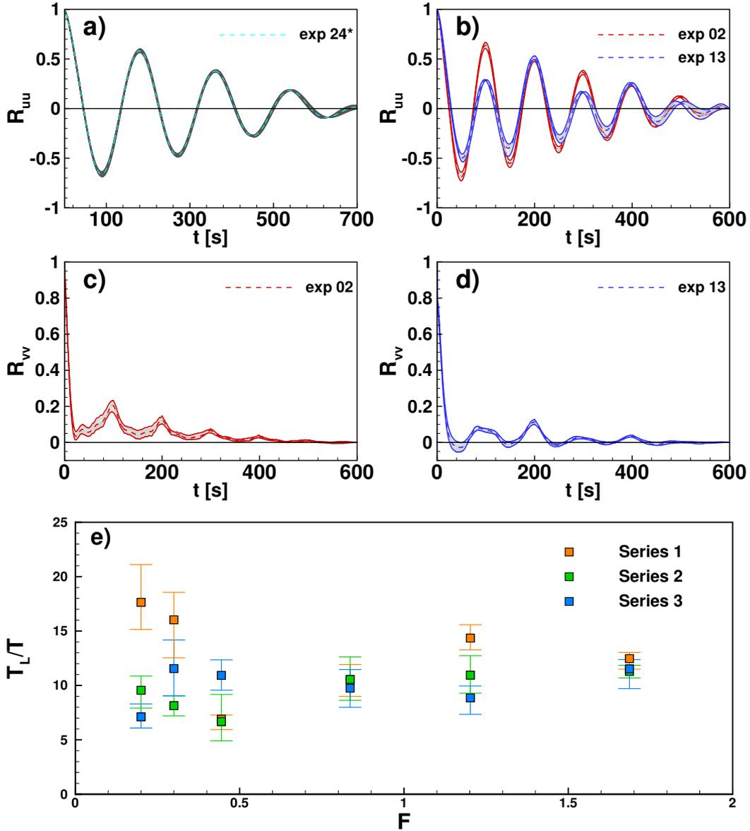
**Figure 6.** Autocorrelation functions. Panel a)  $R_{uu}$  experiment 24 of De Leo et al. Panel b)  $R_{uu}$  experiments 2 and 13. Panel c)  $R_{vv}$  experiment 2. Panel d)  $R_{vv}$  experiment 13. Panel e) non dimensional Lagrangian integral scales as a function of the form factor  $F$ . Squared symbols stand for averaged values whereas bars for their spreads.
