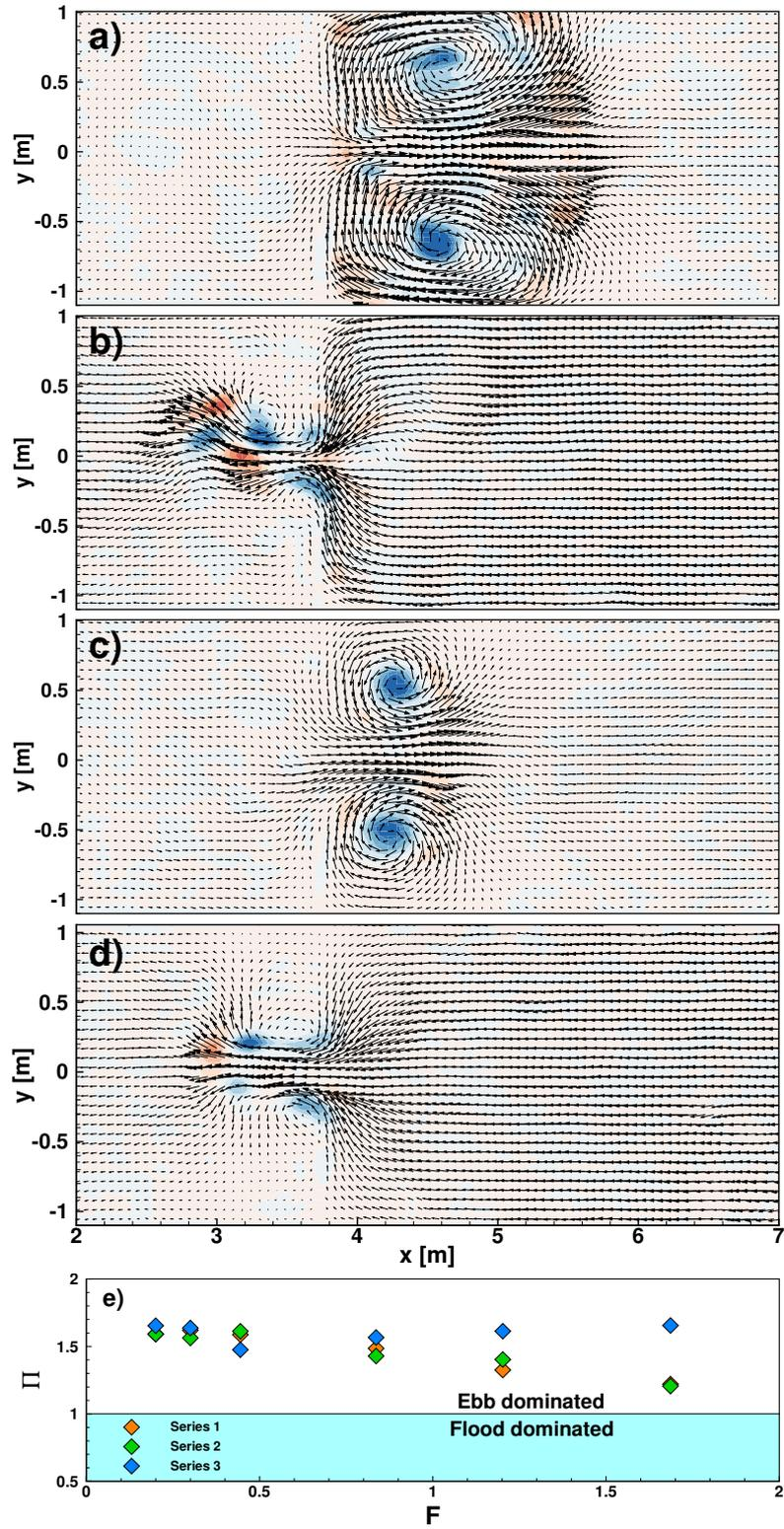
**Figure 4.** Examples of time dependent two dimensional velocity fields with Okubo-Weiss parameter contours for experiment 5. Panel a) maximum crest flood phase; panel b) and d) flushing ebb phase; panel c) less intense flood. Panel e) Power ratio of ebb and flood powers computed as the time integral of the kinetic energy per unit mass as a function of the form factor  $F$
