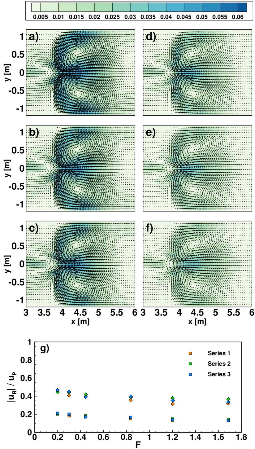
**Figure 5.** Panel a) to f): examples of residual currents fields for experiments of series 1. g): average residual velocity (squares) and maximum residual velocity (diamonds) divided by the tidal velocity peak at the inlet ( $|u_p|$ ) as function of the form factor  $F$ .
