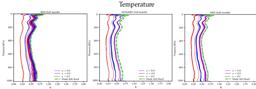
**Figure 11.** Vertical standard deviation profiles of Temperature for periods (left to right); M18, M18sM03 and M03. Standard deviations of; BS (green-dotted-line), B8020  $\alpha = 0.8$  (purple lines), B5050  $\alpha = 0.5$  (blue-lines) and B2080  $\alpha = 0.2$  (red-lines).
