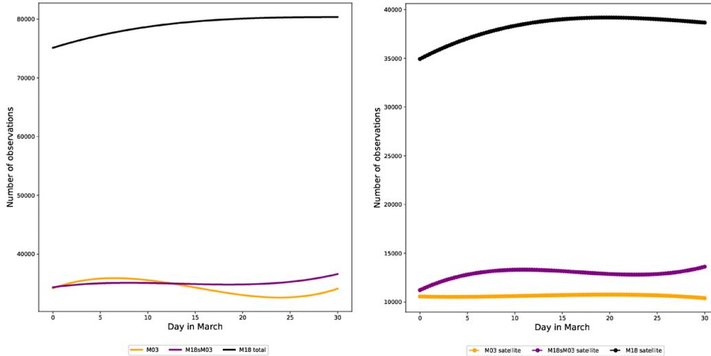
**Figure 6.** Total numbers of observations (left plot) and satellite observations (right plot), by day in March (x-axis), for: March-2003 (orange line), March-2018 simulating March-2003 observations and March-2018 with default settings (black line). The observation data was averaged using a 4<sup>th</sup> degree polynomial.
