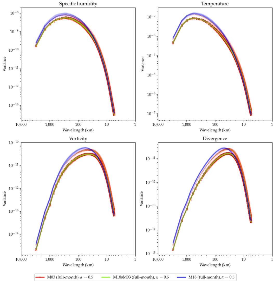
**Figure 10.** Horizontal variance spectra at 1000hPa of; specific humidity (top-left), temperature (top-right), vorticity (bottom-left) and divergence (bottom-right) of forecast errors for B-matrix B5050 during periods; M03 (red-lines), M18sM03 (teal-lines), M18 (blue-lines).
